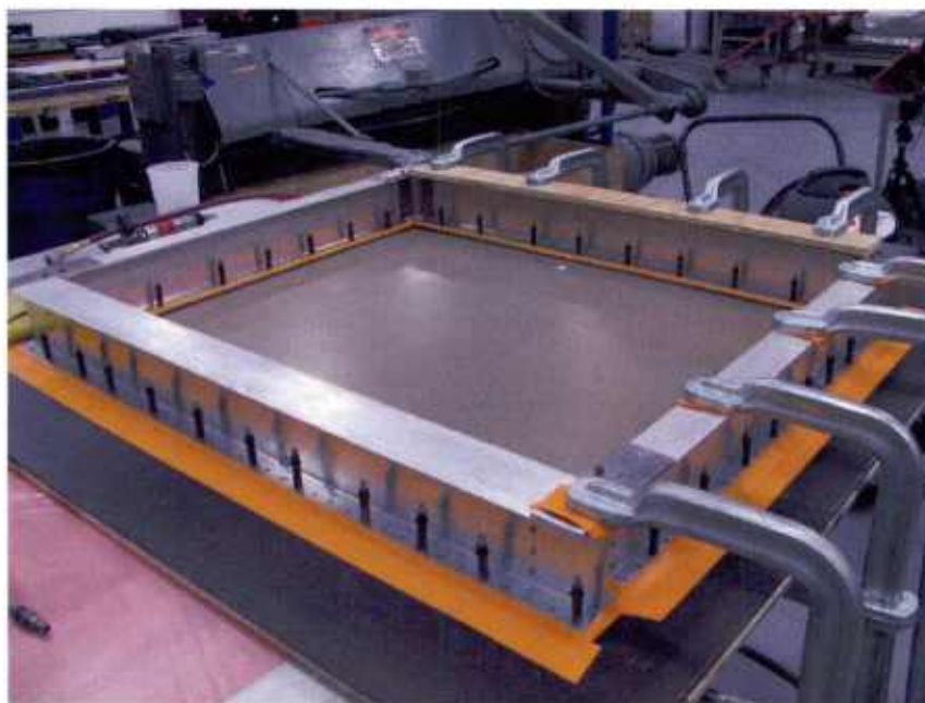
Figure 91. Match drilled holes for framing.
