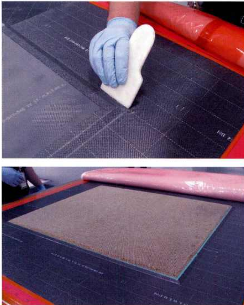
Figure 89. Top – hand working of edge material, Bottom – application of honeycomb core.
