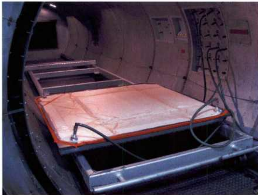
Figure 90. Top – Completed single subpanel, Bottom – Curing of vacuum-sealed subpanel.
