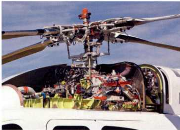
Figure 1. View of the inside of the transmission region in a commercial rotorcraft.
