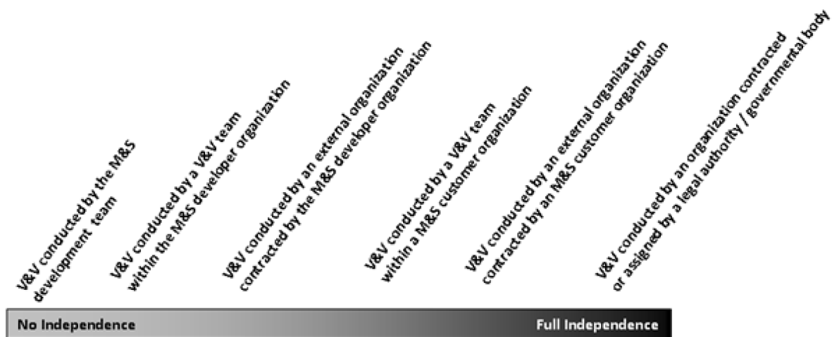
Figure 4-6: Levels of Independent V&V.
