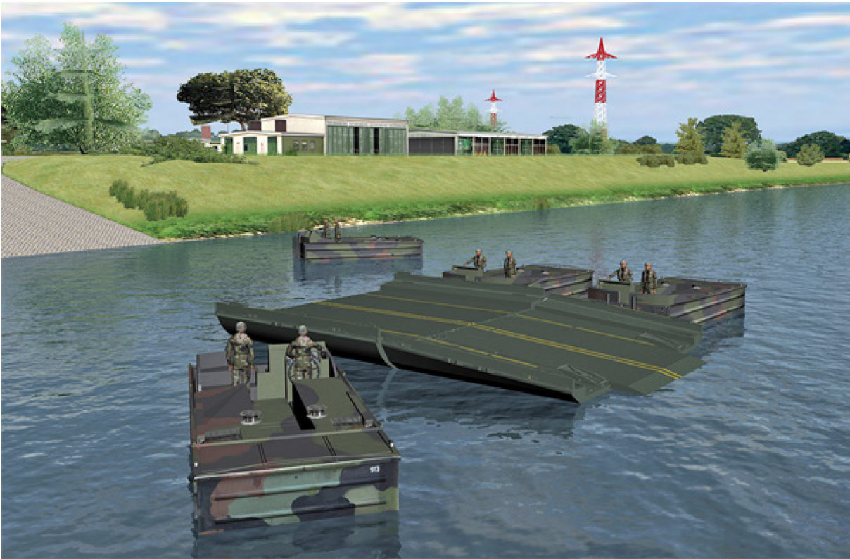
Figure 8-1: Pioneers Ribbon/Floating Bridge.
