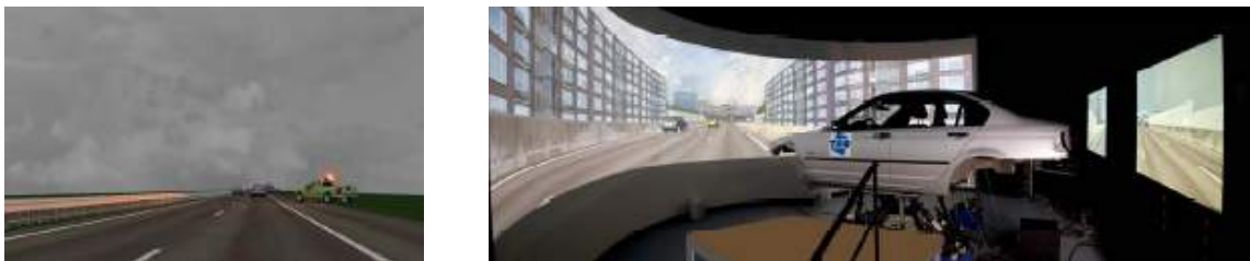
Figure 7-1: The TNO Driving Simulator.
