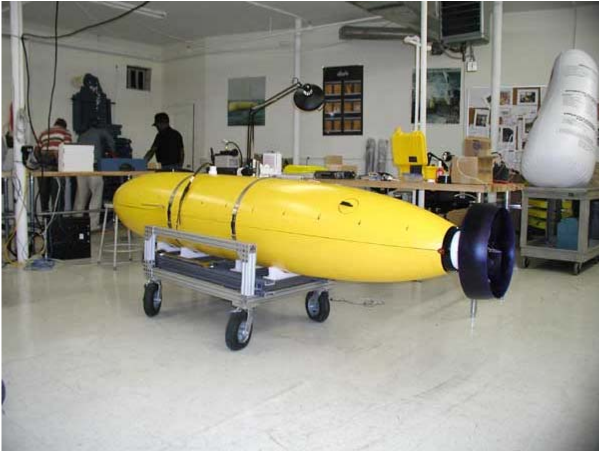
Figure 1. A Bluefin Robotics Odyssey III AUV with a configuration similar to that on order for Oregon State University.
