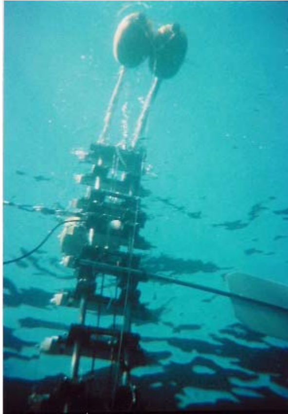
Figure 1. Vertical array surface sampler (VASS) pictured under water. 12 individual sample bottles (0-2.2m, \Delta z=0.2m ) are simultaneously triggered electrically.
