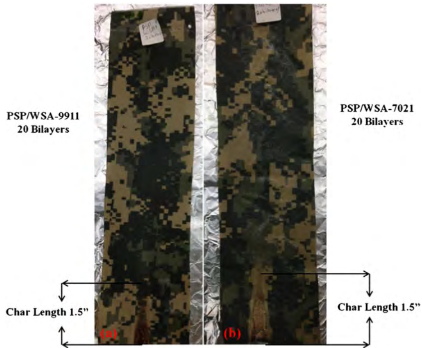
Figure 8. Post vertical flame test images of (a) PSP/W SA-9911 and (b) PSP/W SA-7021 with char length of 1.5" (3.81 cm).
