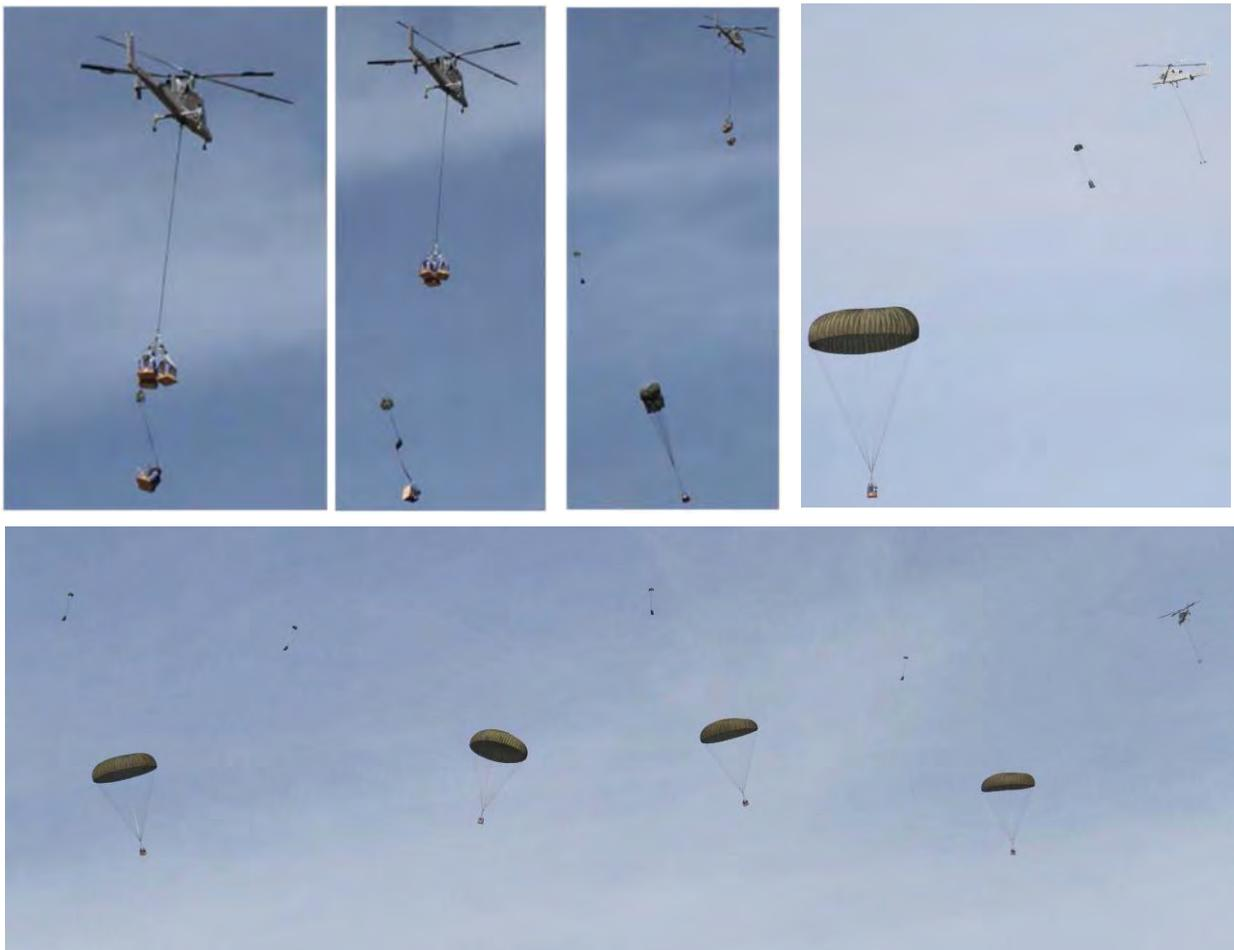
Figure 10: Container Delivery System (CDS) Inflation Sequence during Third K-MAX Demonstration (25 Jan 2011)
