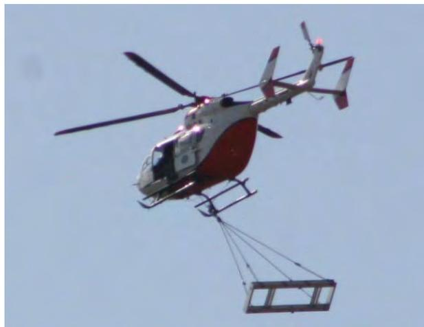
**Figure 34: Quarter System High-Speed UH-72 Flight with Empty System**
