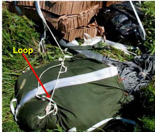
Figure 50: Loop Created during Second UH-72 Airdrop Test Week
