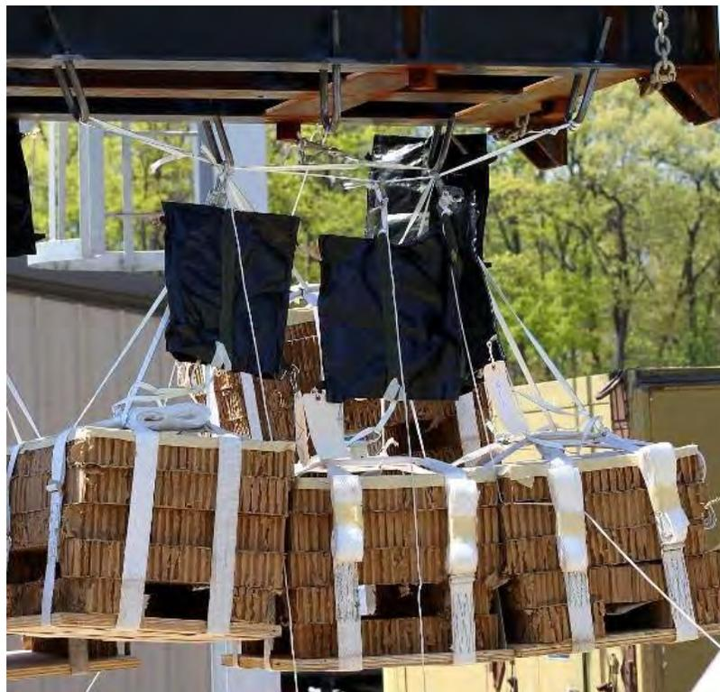
Figure 11: Single-Cable Suspension
