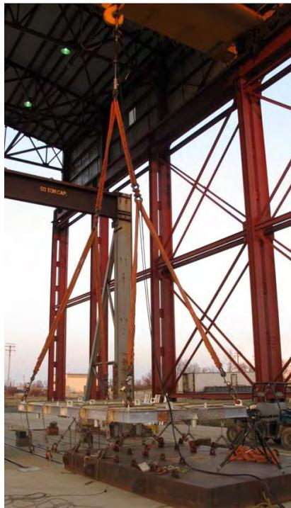
Figure 32: Full System Proof Load Test Setup
