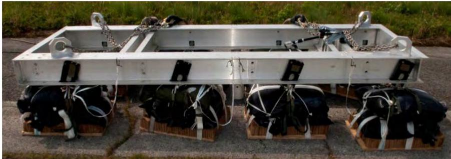
Figure 48: Payloads Attached to Frame for Second UH-72 Airdrop Test Week (10-12 July 2012)
