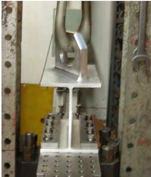
Figure 24: Lift Provision Tensile Testing Setup
