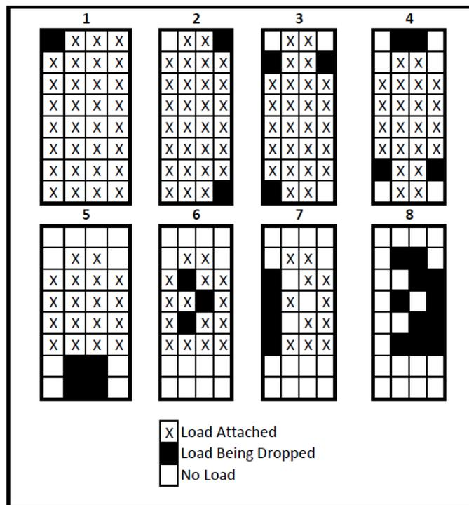
Figure 55: CH-47D Test Airdrop Order (13-23 May 2014)
