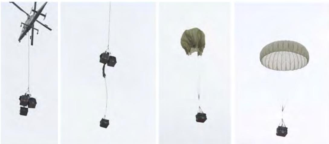
Figure 8: Inflation Sequence of One T-10 Cargo Parachute during Second K-MAX Demonstration (14-15 Nov 2010)
