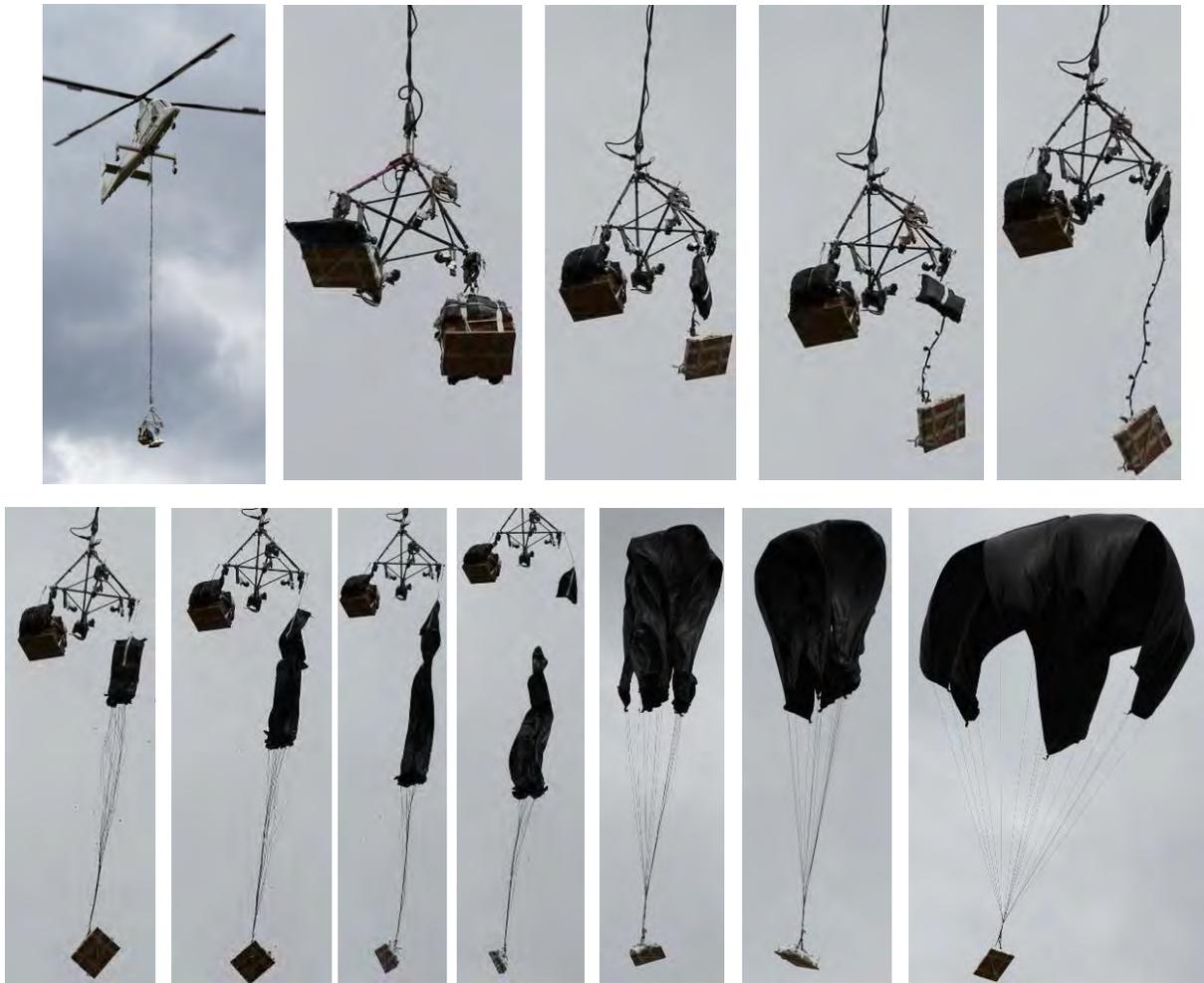
**Figure 5: Inflation Sequence of LCLA Parachute during First K-MAX Demonstration (21-22 Apr 2010)**
