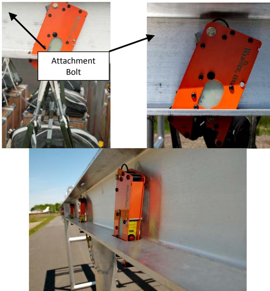
Figure 21: WGRMs Attached to HSL RADE Frame
