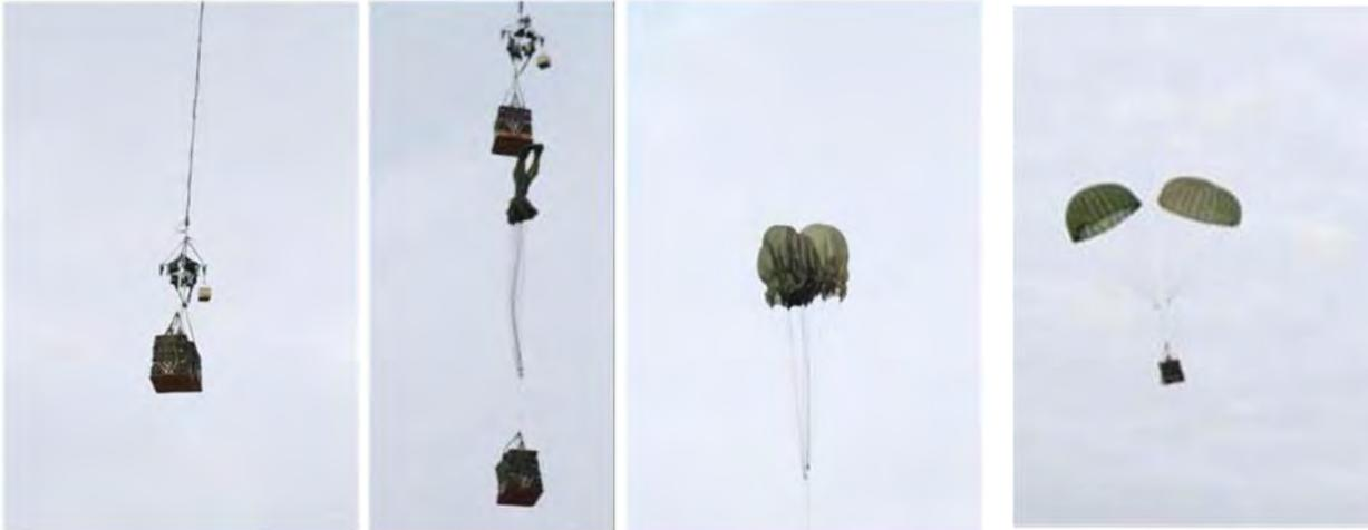
Figure 7: Inflation Sequence of Two T-10R Cargo Parachutes during Second K-MAX Demonstration (14-15 Nov 2010)
