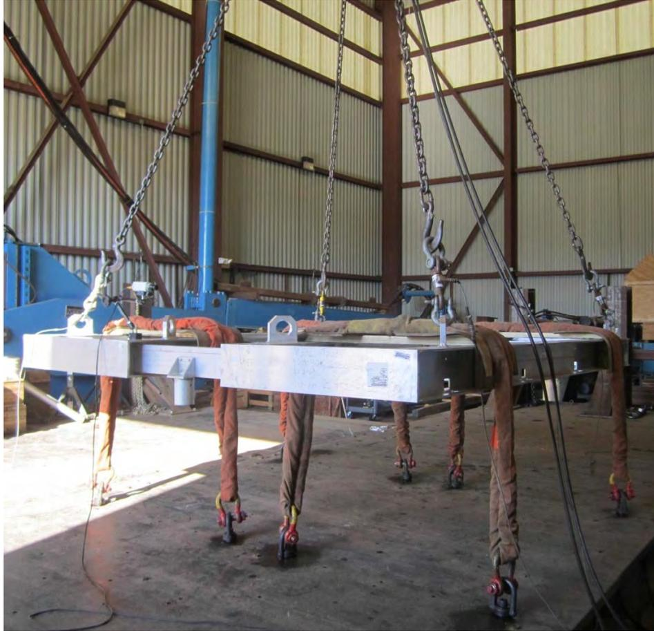
Figure 27: Proof Load Test Setup
