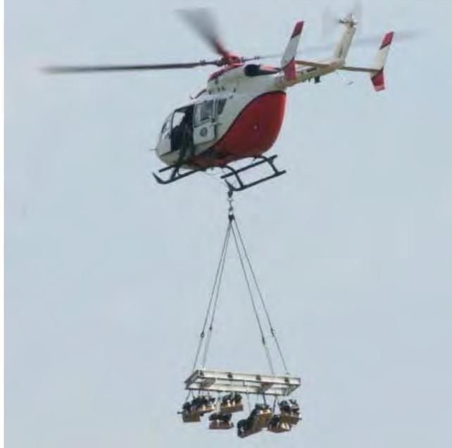
**Figure 33: Quarter System High-Speed UH-72 Flight with Eight Payloads**
