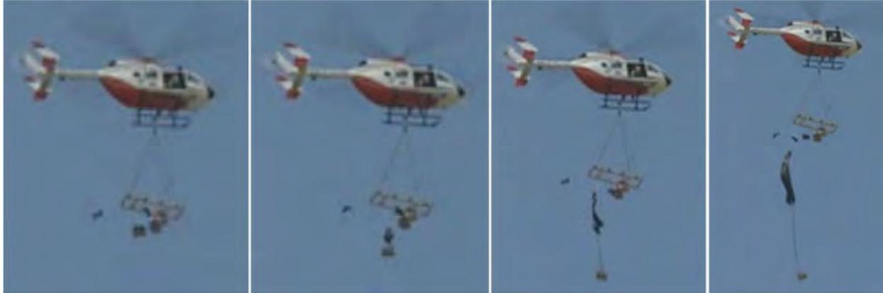
Figure 41: Inflation Sequence of LCLA Parachute from HSL RADE
