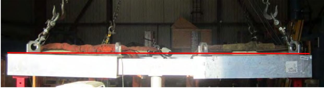
Figure 28: Half System Proof Load Test Setup
