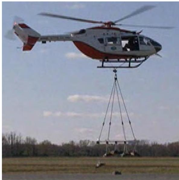
Figure 36: Helicopter Payload Release Test
