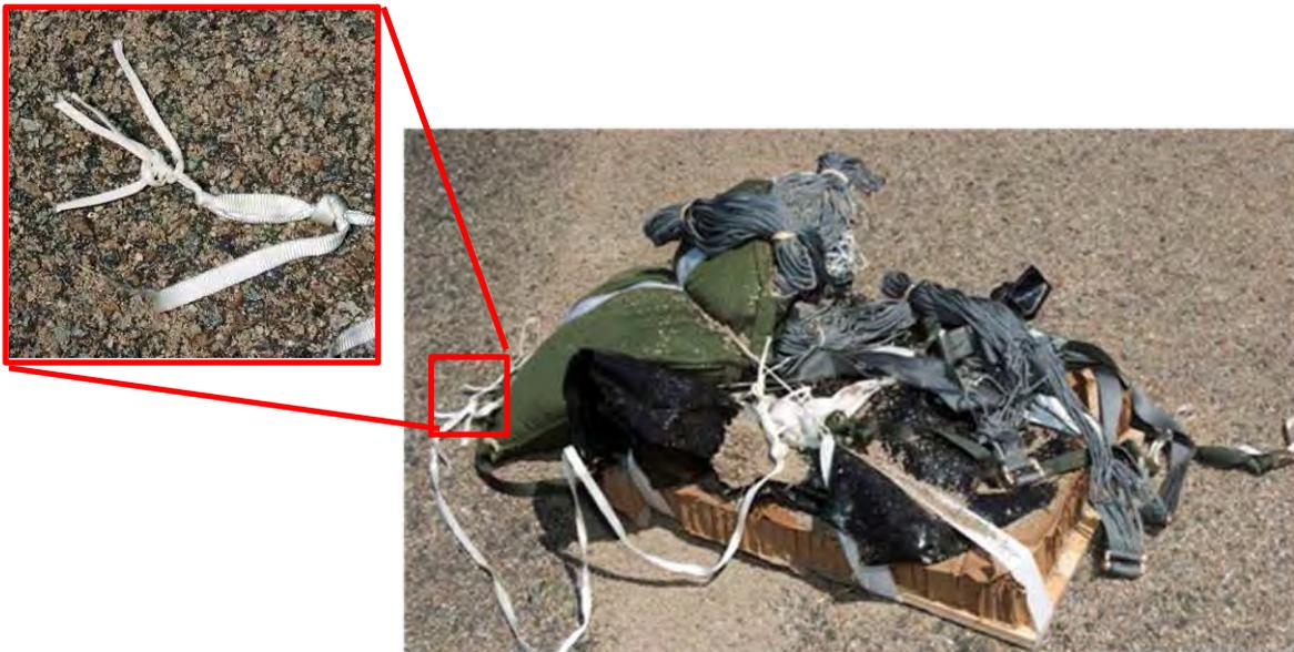
Figure 42: T-10 Cargo Broken Static Line
