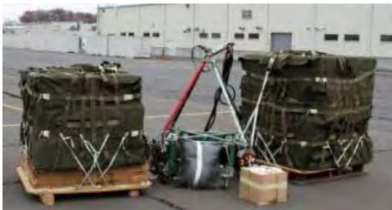
**Figure 6: Final Rigged Configuration of A-22 Containers for Second K-MAX Demonstration (14-15 Nov 2010)**
