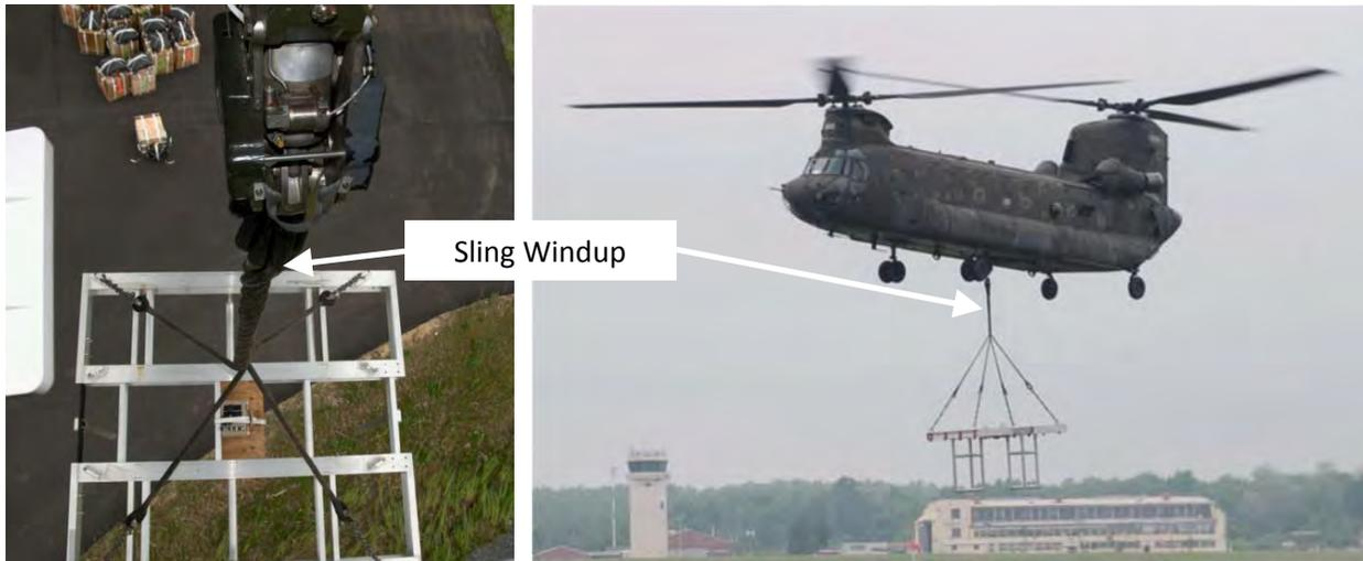
Figure 54: Half Frame Instability during CH-47D Airdrop Tests (13-23 May 2013)
