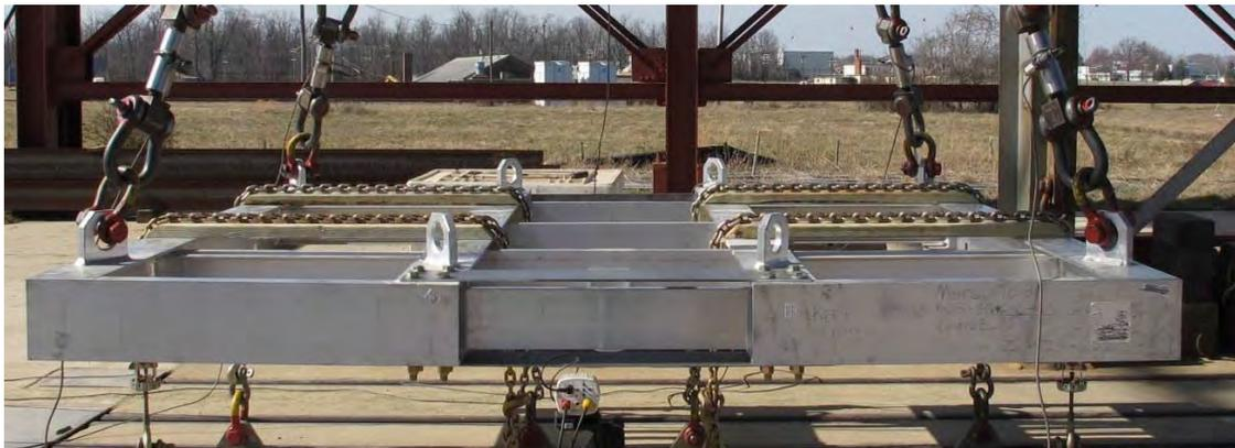
**Figure 30: Half System Proof Load Test Setup with Steel Plates**
