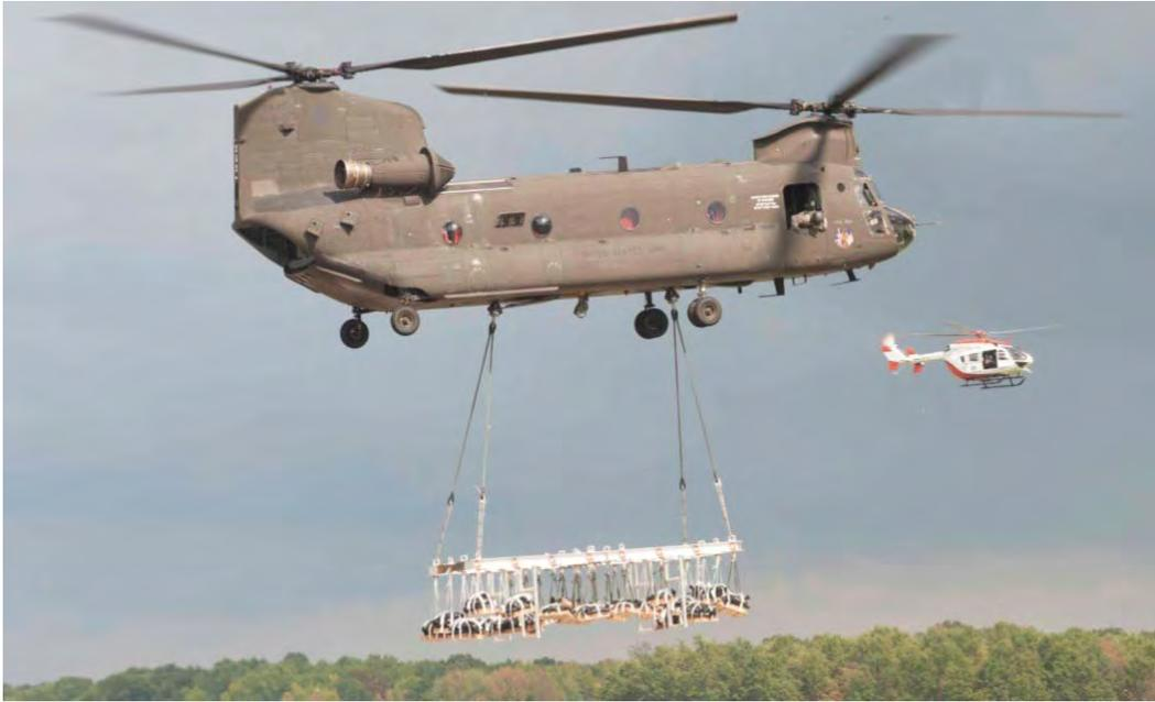
Figure 35: Full HSL RADE System under CH-47 Helicopter
