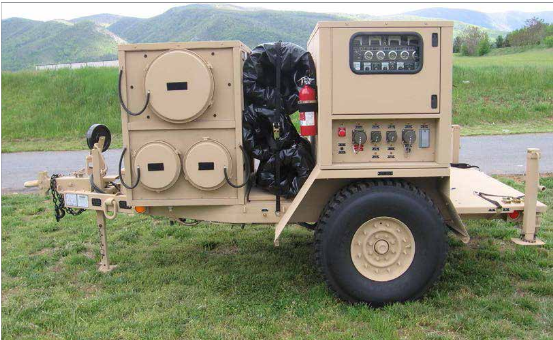
GET Trailer system showing airflow ducts on the left side and control panel on the right side.
