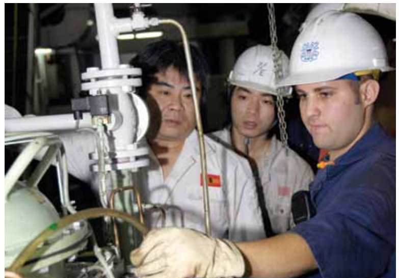
A U.S. Coast Guard port state control examiner checks the oily water separator system on a foreign vessel. U.S. Coast Guard photo by Petty Officer Brandyn Hill.
