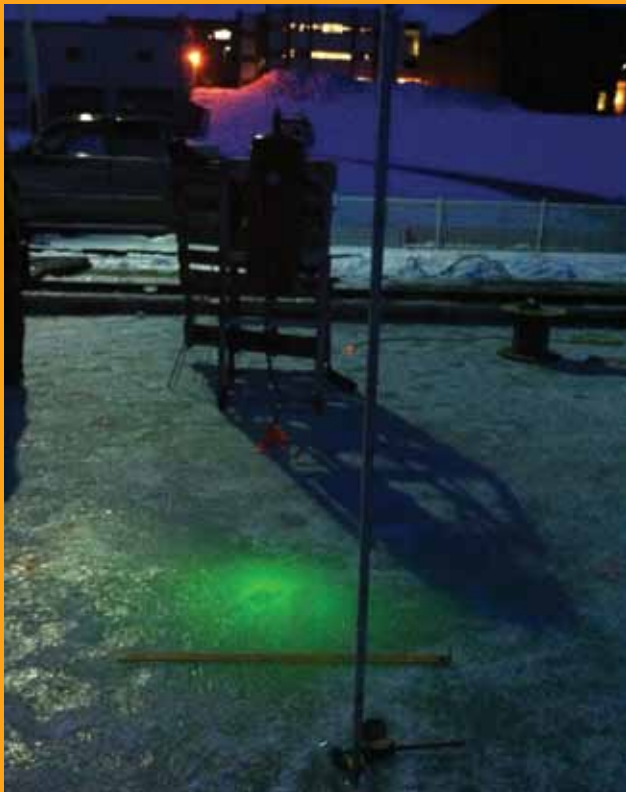
Night testing for submerged oil detection systems at the Cold Regions Research and Engineering Laboratory's geophysical research facility. Photo courtesy of Mr. J. Wilkinson, Scottish Association of Marine Science.
