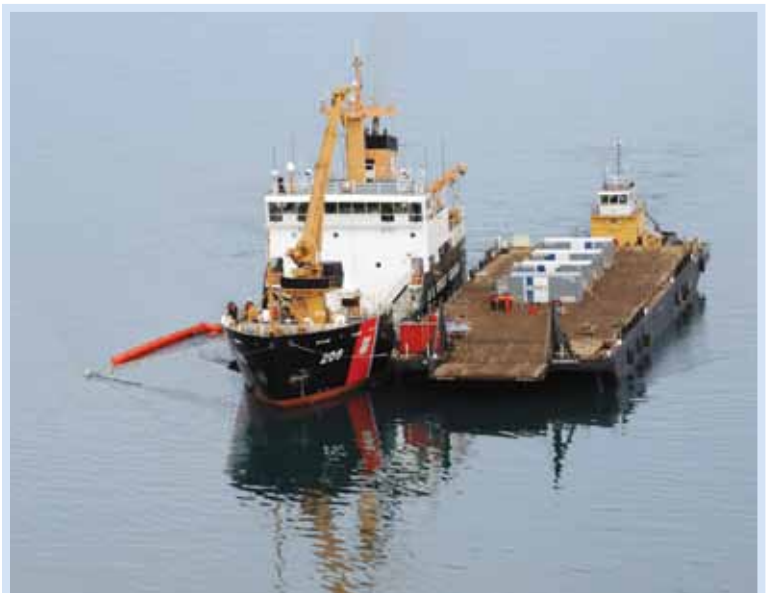
Coast Guard Cutter Sycamore crewmembers deploy the cutter's spilled oil recovery system equipment near Barrow, Alaska. U.S. Coast Guard photo by Petty Officer Kelly Parker.
