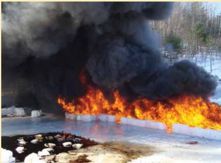
As part of the hands-on training, oil burns in a recovery trench at CRREL's Geophysical Research Facility. In situ burning is considered one of the most effective means to mitigate an oil spill.
