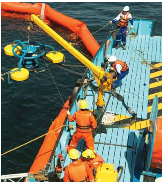
A vessel crew deploys a skimmer off the coast of Brazil. Photo courtesy of Elastec/American Marine.
