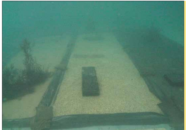
The Ohmsett facility uses a test tank filled with sand, rocks, oil, and seaweed to test recovery methods. U.S. Coast Guard RDC photo.
