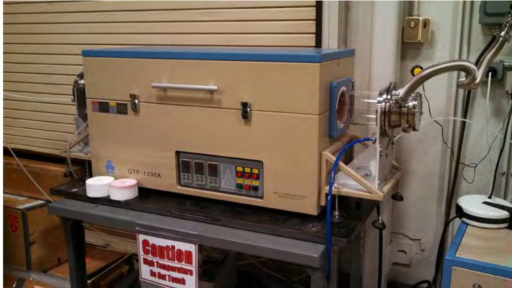
Fig. 1 Chemical vapor deposition (CVD) furnace showing vacuum lines and temperature controller
