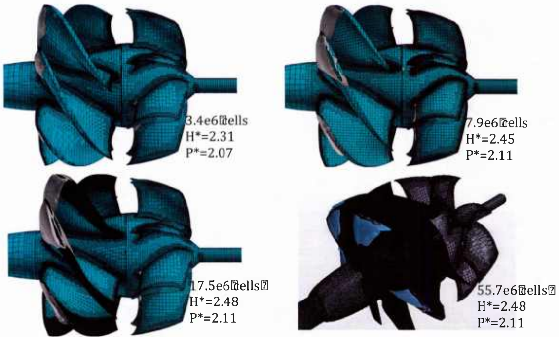
Figure 4: Sensitivity of unsteady cavity resolution to computational mesh. Solution (d) is still evolving.
