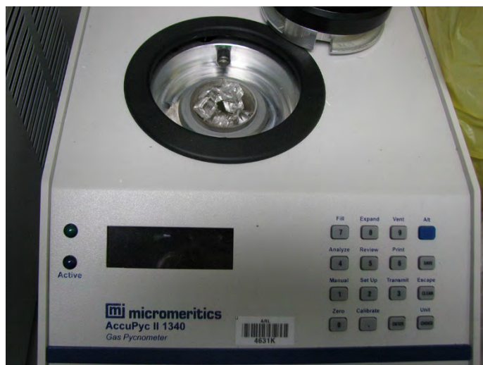
Fig. 1 Sample cup in the sample chamber to be sealed by the chamber cap (upper right)
