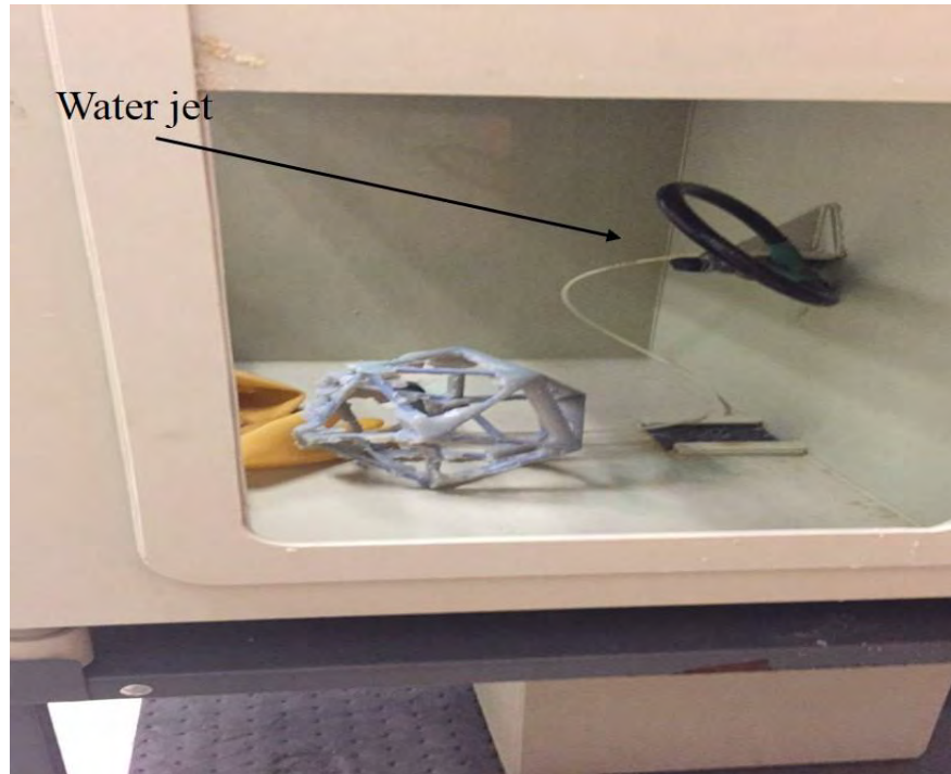
Figure 18: Water jet cleaning off the support material
