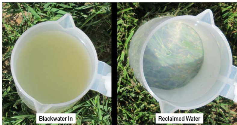
Figure 6.5. Photos of blackwater entering the Living Machine and reclaimed water.
