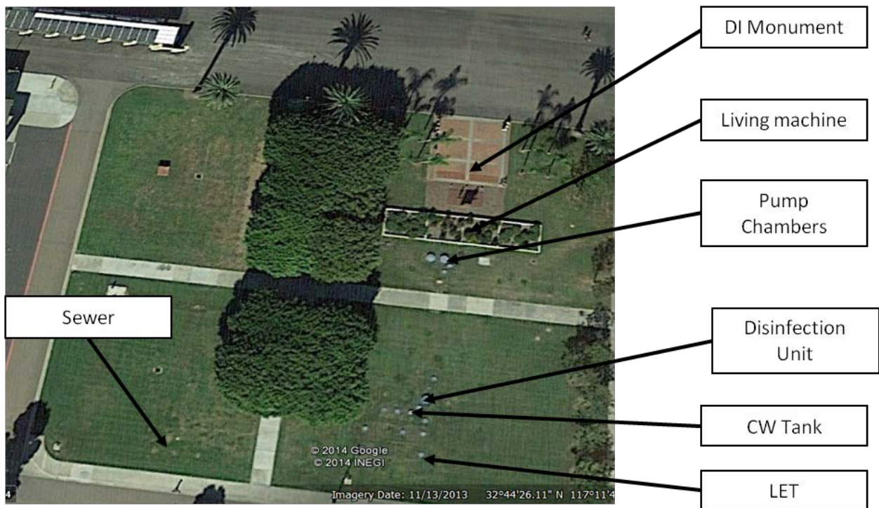
Figure 5.6. Aerial view (Google Earth 13 November 2013) shows the completed installation.
