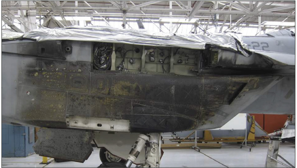
Figure 5: F/A-18 Super Hornet Aircraft with Fire Damage
