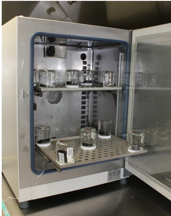
Figure 17. Temperature-mapping probe locations within the test chamber.
