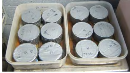
Figure 6.13 Sorption test specimens with one surface exposed to water.
