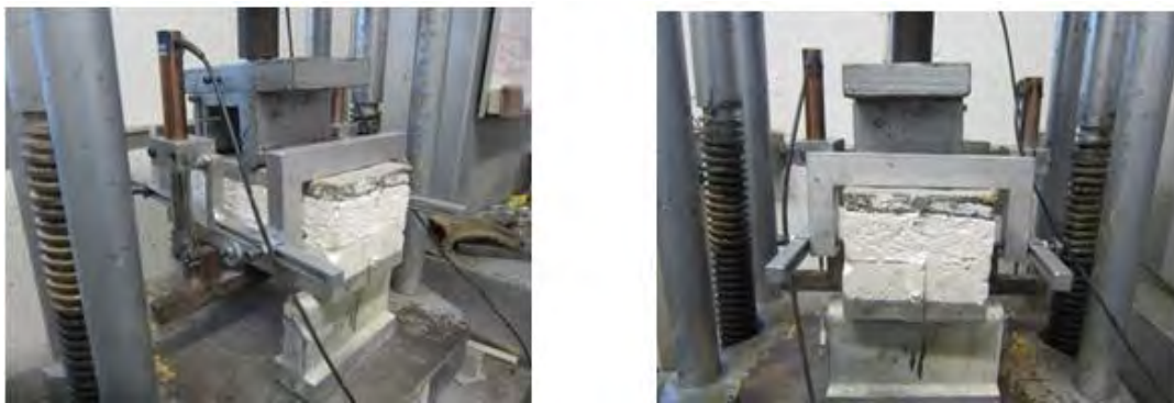
Figure 7.2 Sandwich composite flexure test setup.
