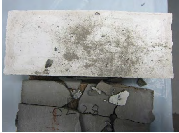
(b) Core surface (top) after removal of delaminated skin
