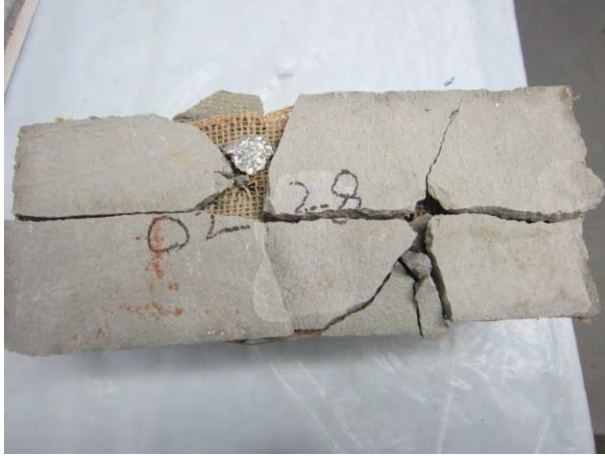
(a) Extensive cracking and delamination of skin
