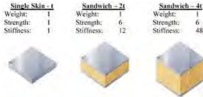
Figure 4.2 Structural efficiency of sandwich composites subjected to flexure.
