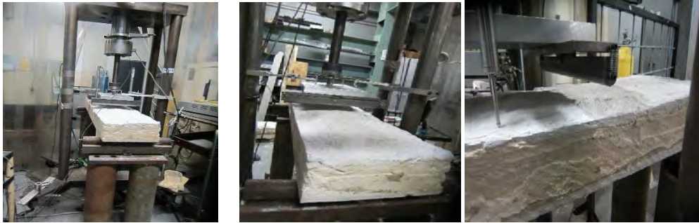
Figure 8.11 Long-span indigenous sandwich composite panel test setup.
