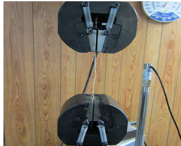
Figure 3.9 Optic microscope image of the jute fiber yarn. Figure 3.10 The single yarn tension test setup.
