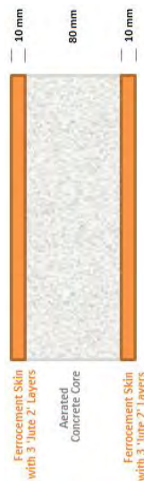
Figure 4.16 A viable sandwich composite design for the B-hut walls.
