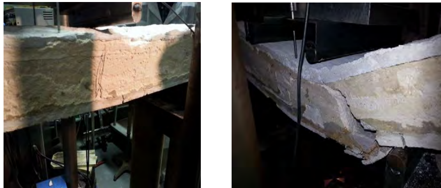
(a) Initial cracking of tension skin (b) Failure mode Figure 8.12 Failure mode of the long-span indigenous sandwich composite panel.
