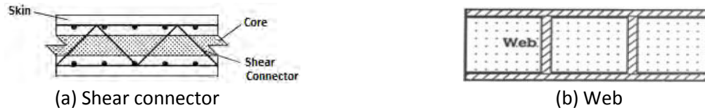
Figure 8.2 The shear connector and web options for ensuring the integrated action of composite skins and the lightweight core in sandwich composites [111].
