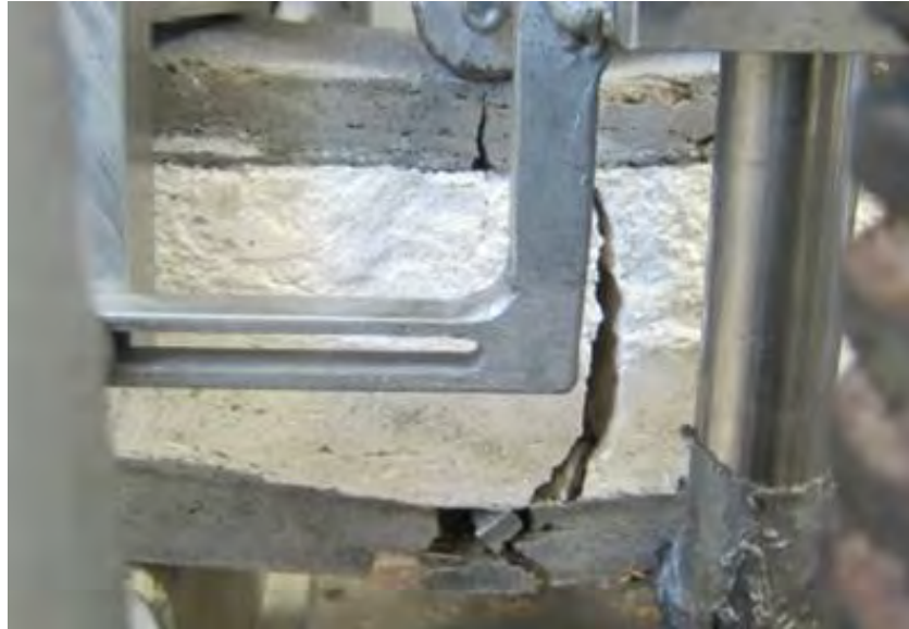
(b) Failure by rupture of the lower skin followed by full-depth cracking of sandwich composite Figure 7.3 Failure mode in flexure of the first-generation sandwich composite.
