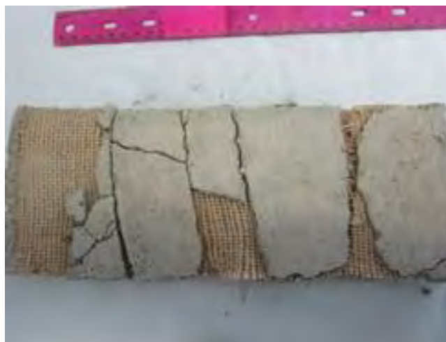
Figure 5.15 Delamination of the mortar coating on the outer layer of the 'Jute 1' burlap with fine opening size.
