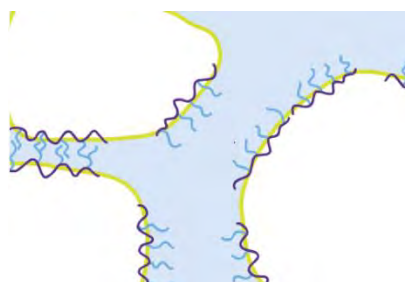
Figure 6.3 Stabilization of larger air bubbles by surfactant molecules which orient themselves on the interfaces of larger air bubbles with water ( http://www.dowcorning.com/content/discover/discoverchem/si-stabilizers.aspx ).
