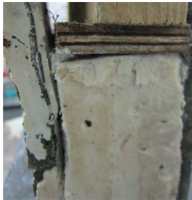
Figure 8.6 Damage mechanism during shear failure of the ferrocement skin-aerated concrete core interface with shear connector.
