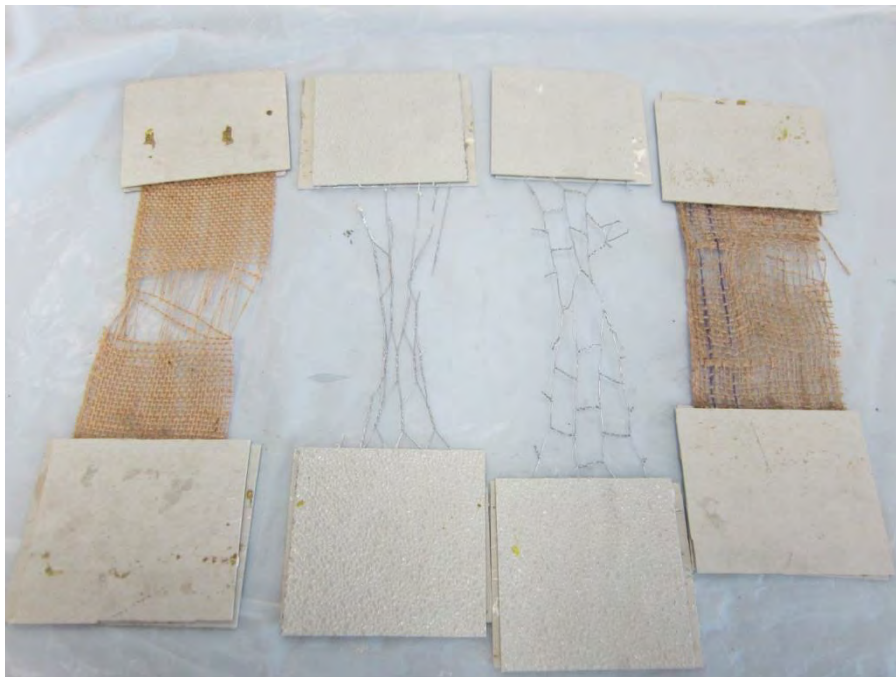
(d) Failed specimens: Jute 1 (left), Chicken mesh in two perpendicular directions (center), Jute 2 (right)
