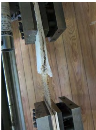
Figure 5.23 Failure by splitting of the ferrocement half of the bond test specimen with 50 mm embedment length.
