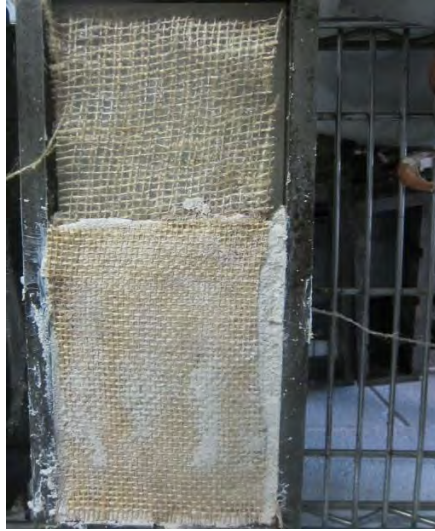
(a) Fabrics placed for preparing the specimen
