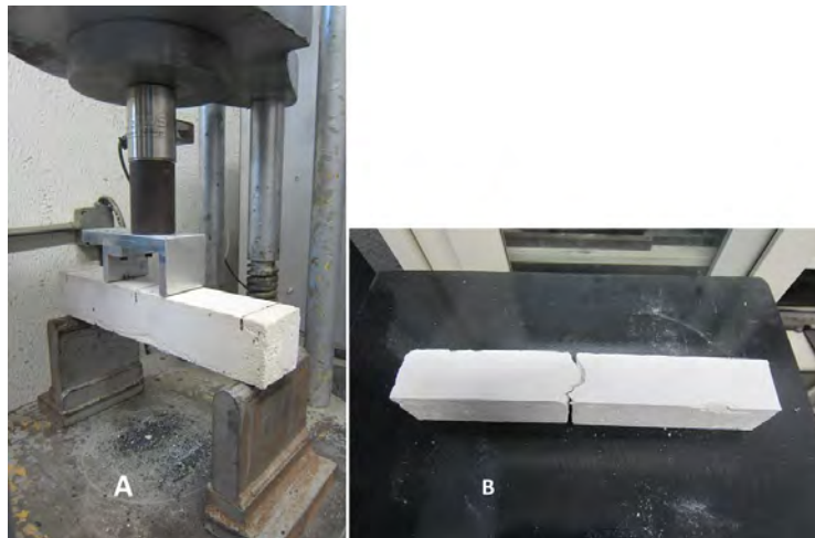
Figure 6.12 Flexural test setup (A) and failure mode (B).
