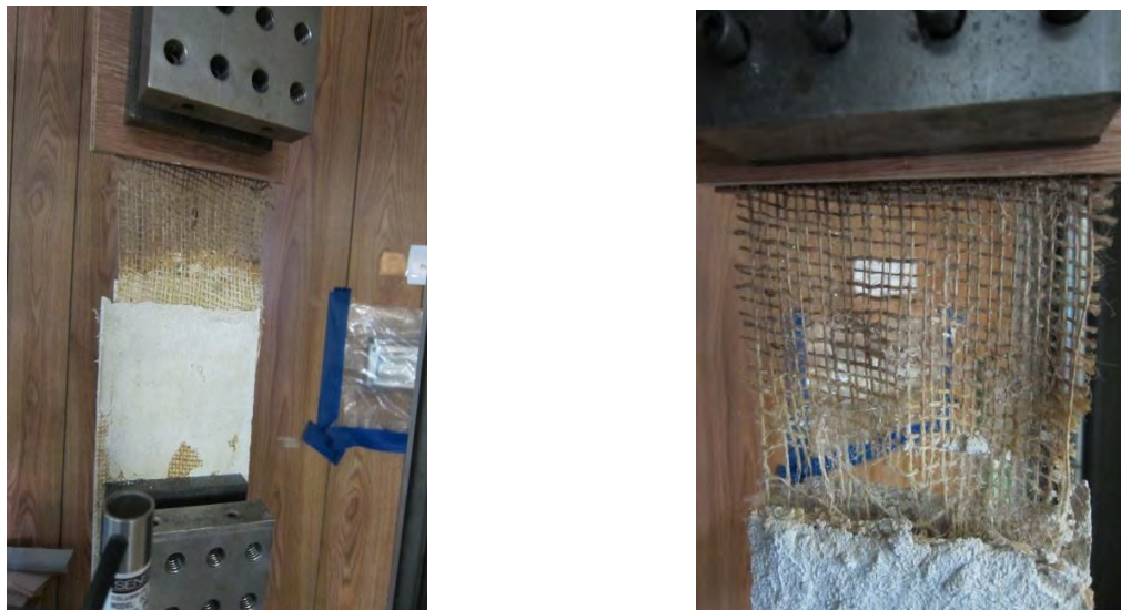
(a) Pullout of fabric with 50 mm embedment length (b) Rupture of fabric with 130 mm embedment length
