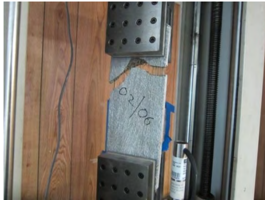
Figure 5.11 Failure of the first-generation ferrocement specimens with formation and growth of a single crack.
