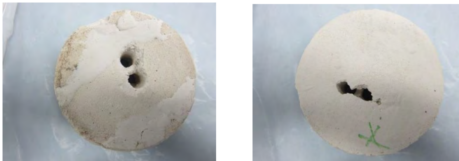
Figure 6.18 Entry and exit points of two projectiles shot at the same specimen.
