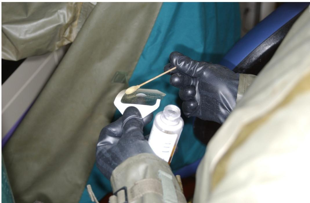
Figure 4. Mastisol application to dosing template.
