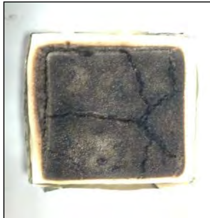
Fig. 2.2 A typical crack pattern that develops after thermal assault
