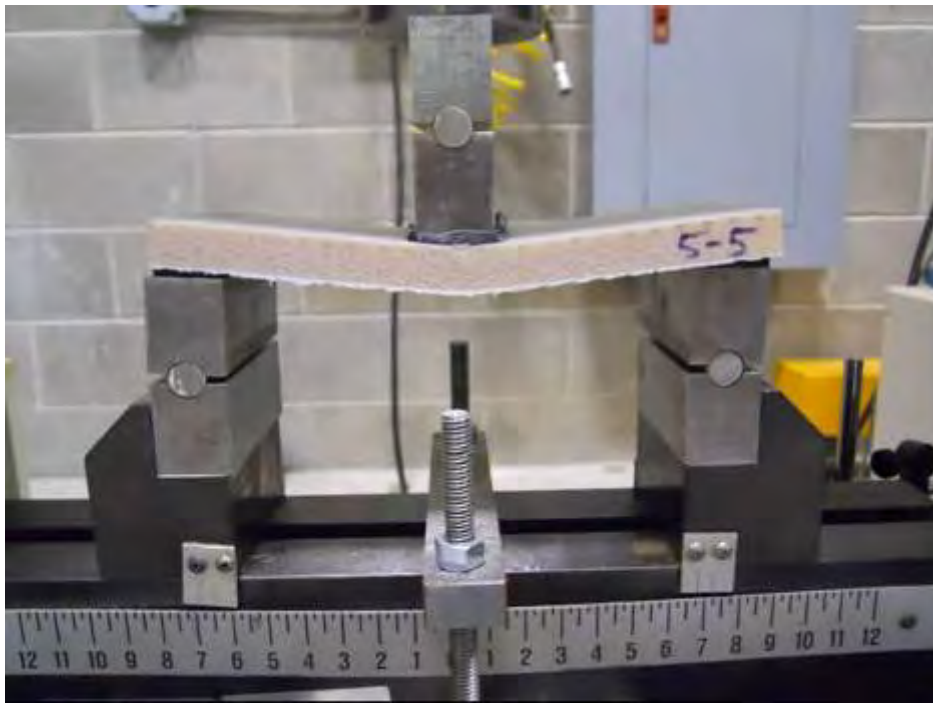
Fig. 9.15 a) 3-point bending experiment for H250, 12.7-mm foam core sandwich panel, and b) sample under load
