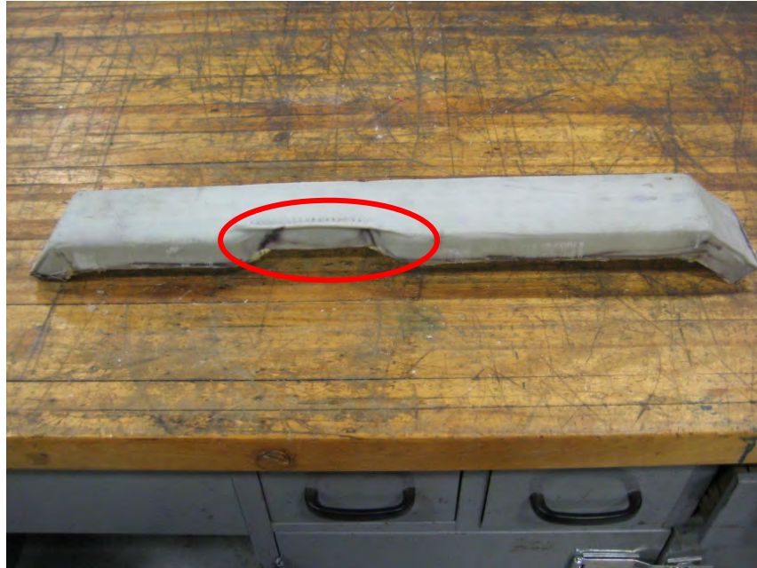
Fig. 9.3.10 Highlighted wrinkle in part surface
