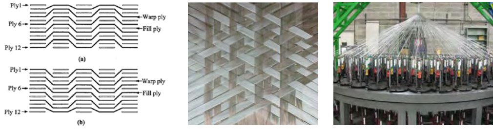
Fig. 7.2.1 Side view of BQ3D woven composite in a) warp and b) fill directions (left), top view of TQ3D woven composite (center), and TQ3D braiding machine (right)
