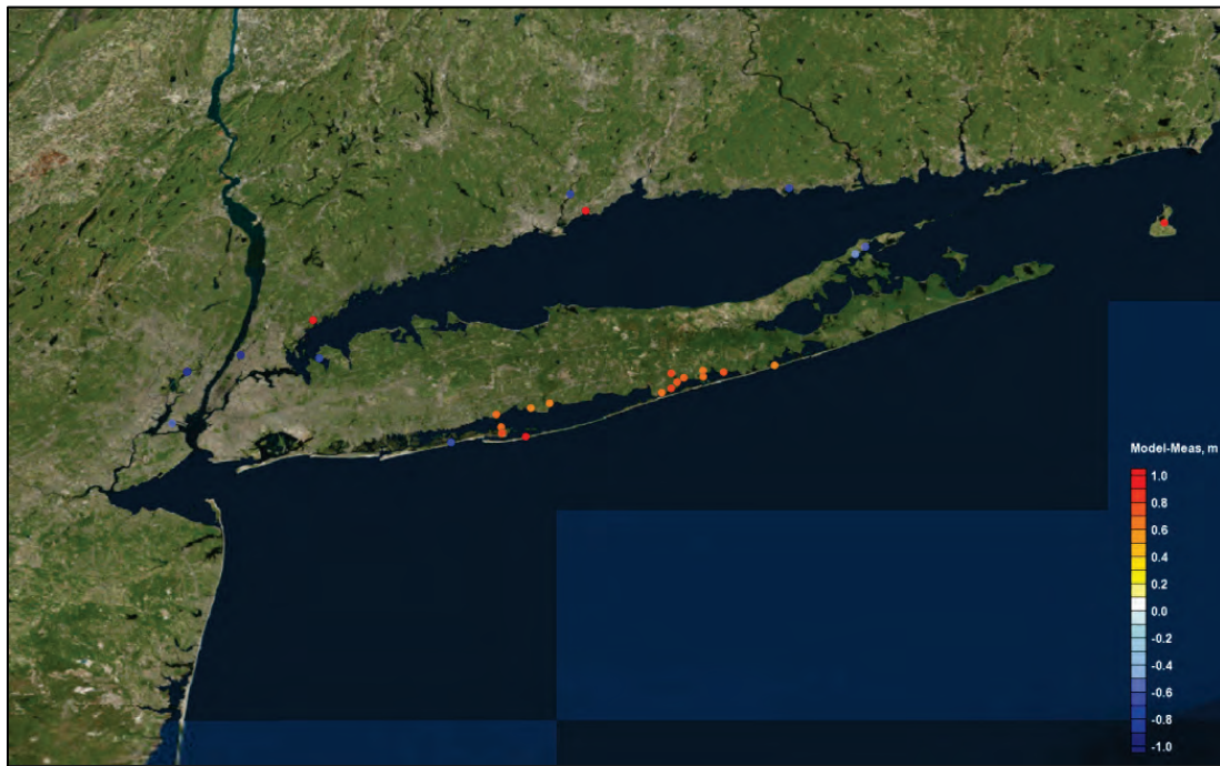
Figure 6-41. Differences between modeled and measured water levels of more than 0.5 m.
