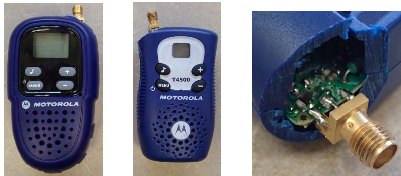
Fig. 3 Targets: FV300 (left), T4500 (center), and connector in place of antenna (right)
