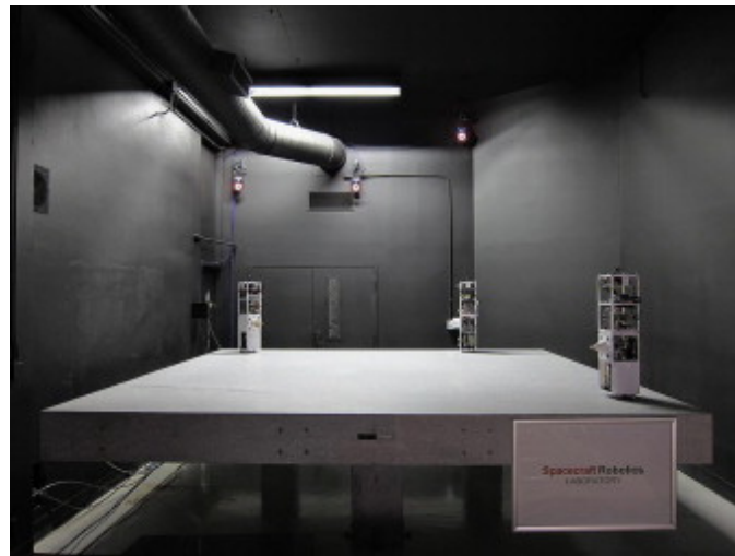
Fig. 14. The Floating Spacecraft-Simulator Testbed at Spacecraft Robotics Laboratory (NPS)
