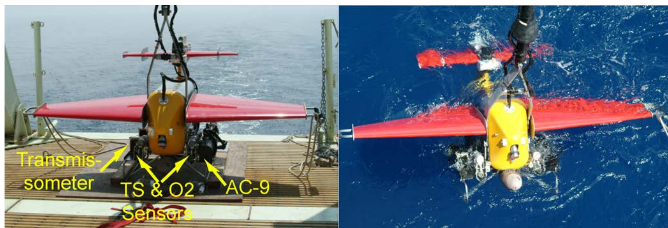
Figure 1. Pictures of the APL/UW Trisoarus tow vehicle equipped with standard CTD sensors as well as the USC WetLabs AC-9 for measuring inherent optical properties. Other sensors are within the body of the vehicle. The picture on the left shows the vehicle on the deck of the ship prior to deployment, and the picture on the right shows the vehicle being deployed in the Adriatic sea..
