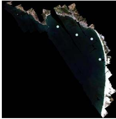
Figure 5: A PHILLS II, three band mosaic of the San Luis Bay, CA site. The locations of ground truth is denoted with the blue dots.
