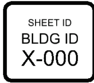
Figure 2-9 Sheet Identification Block.
