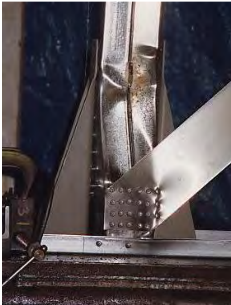
Figure 7-21. Bottom of left column of the A3c panel, showing column deformation and screw rotation.
