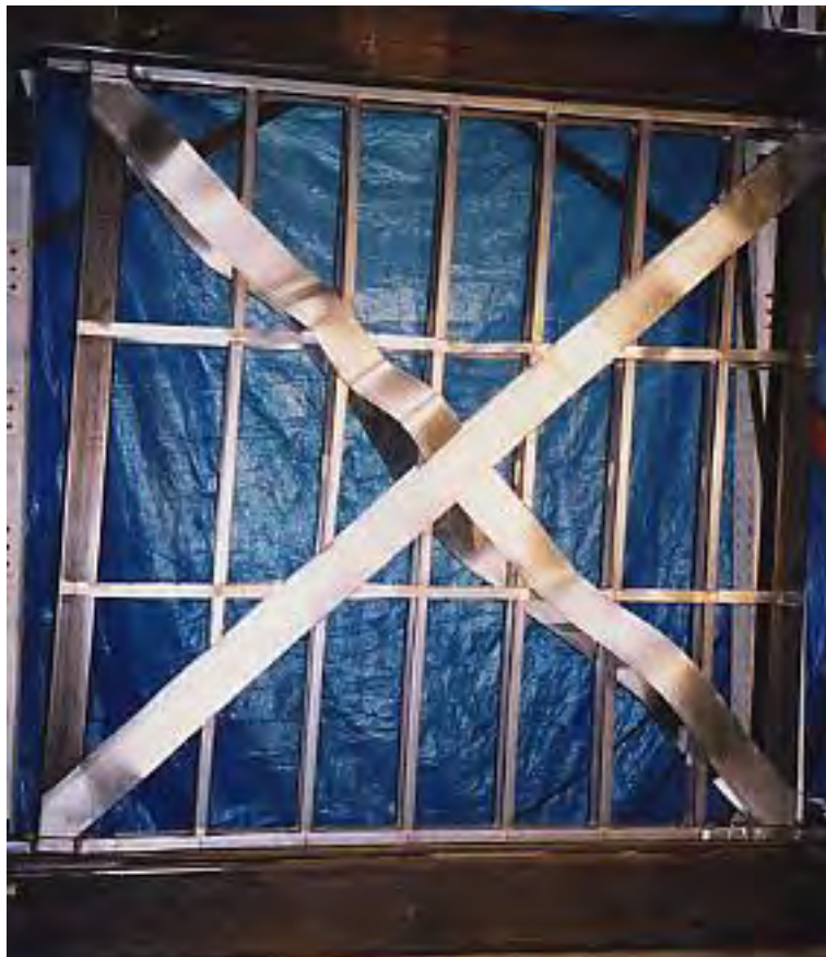
Figure 7-31. Overall view of the D1b test panel at several inches of lateral deflection.
