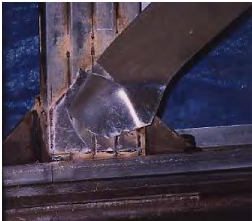
Figure 7-23. Front face of the bottom of the south (left) column, showing strap tearing in the C1a panel.
