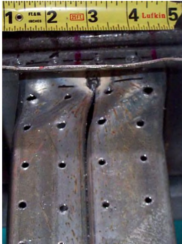
Figure 7-6. Top of right (north) column after A1c panel test.
