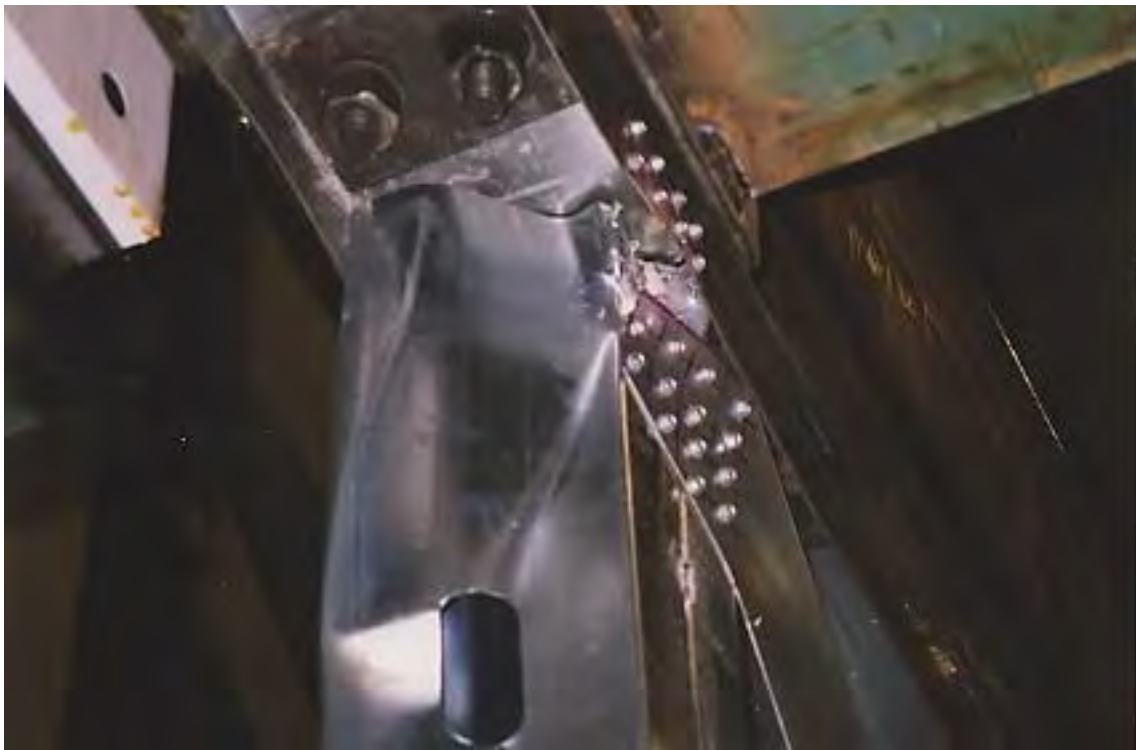
Figure 7-3. Close-up view of column-to-track screw connection failure and column twisting in panel A1-a monotonic test.
