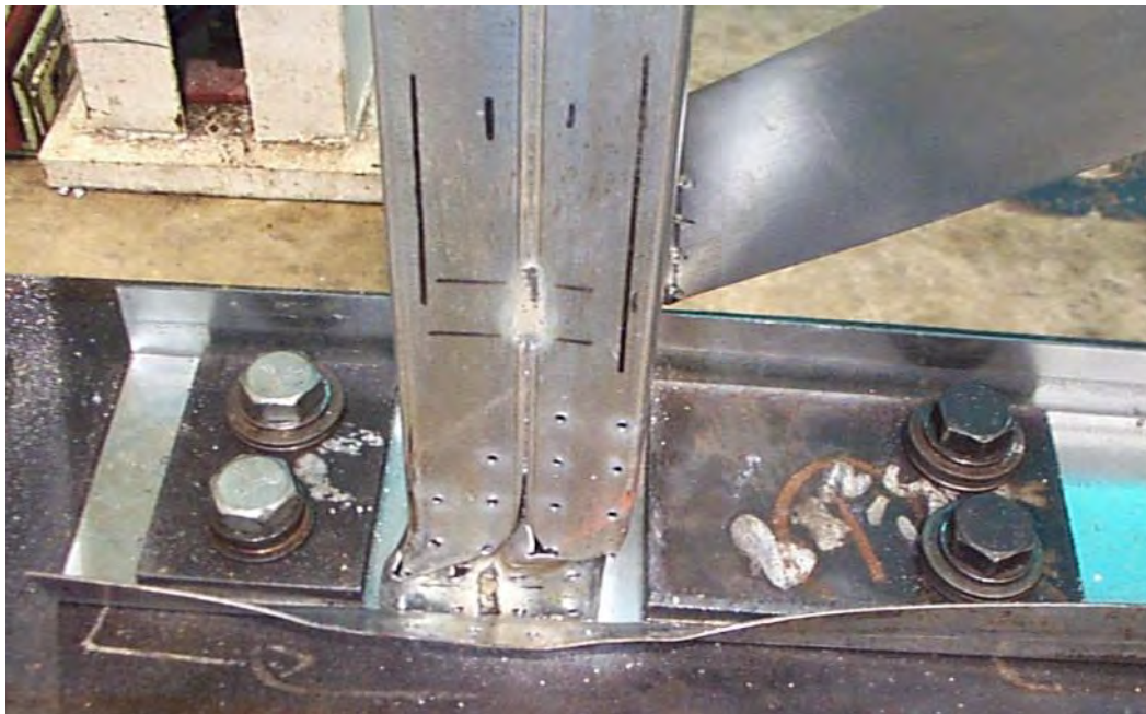
Figure 7-9. Bottom of left (south) column after A1c panel test.
