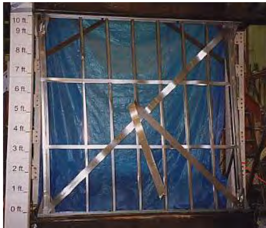
Figure 7-17. Overall view of A3a monotonically tested panel after it failed in the positive direction.
