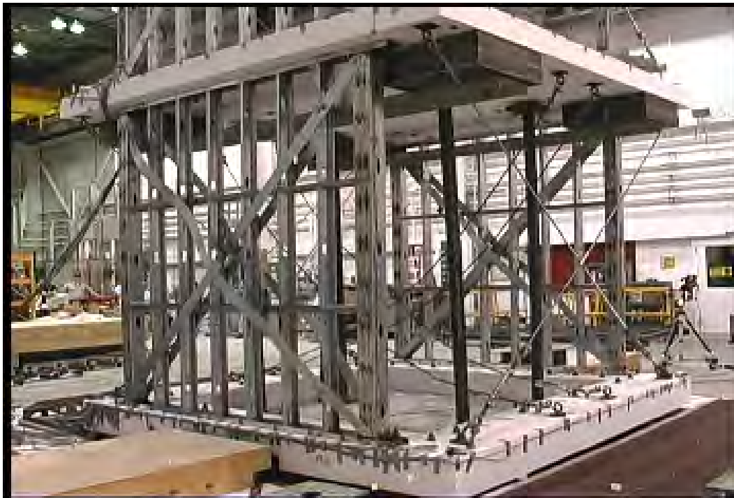
Figure 8-54. First-story view at largest positive cycle, 100% SE32 test near 15.7 sec.
