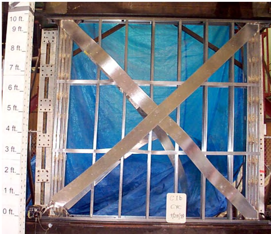
Figure 7-26. Overall view of the C1b panel after failure of three straps and column.
