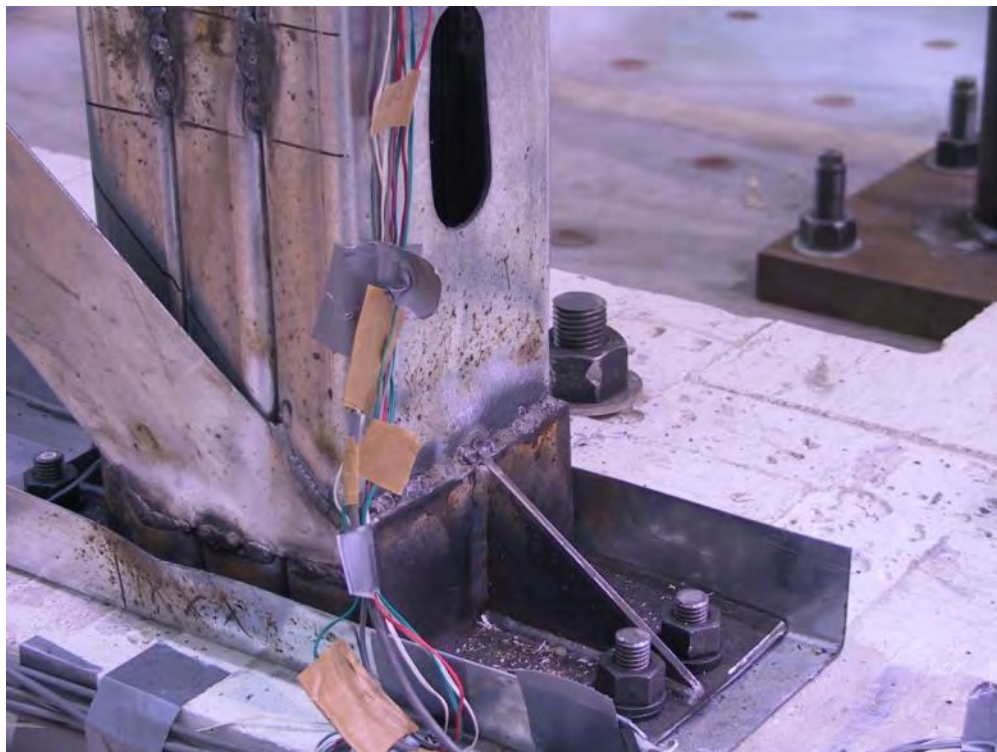
Figure 8-68. Bottom of southwest column facing northeast, showing local column buckling and anchor and column bending at top of the anchor.
