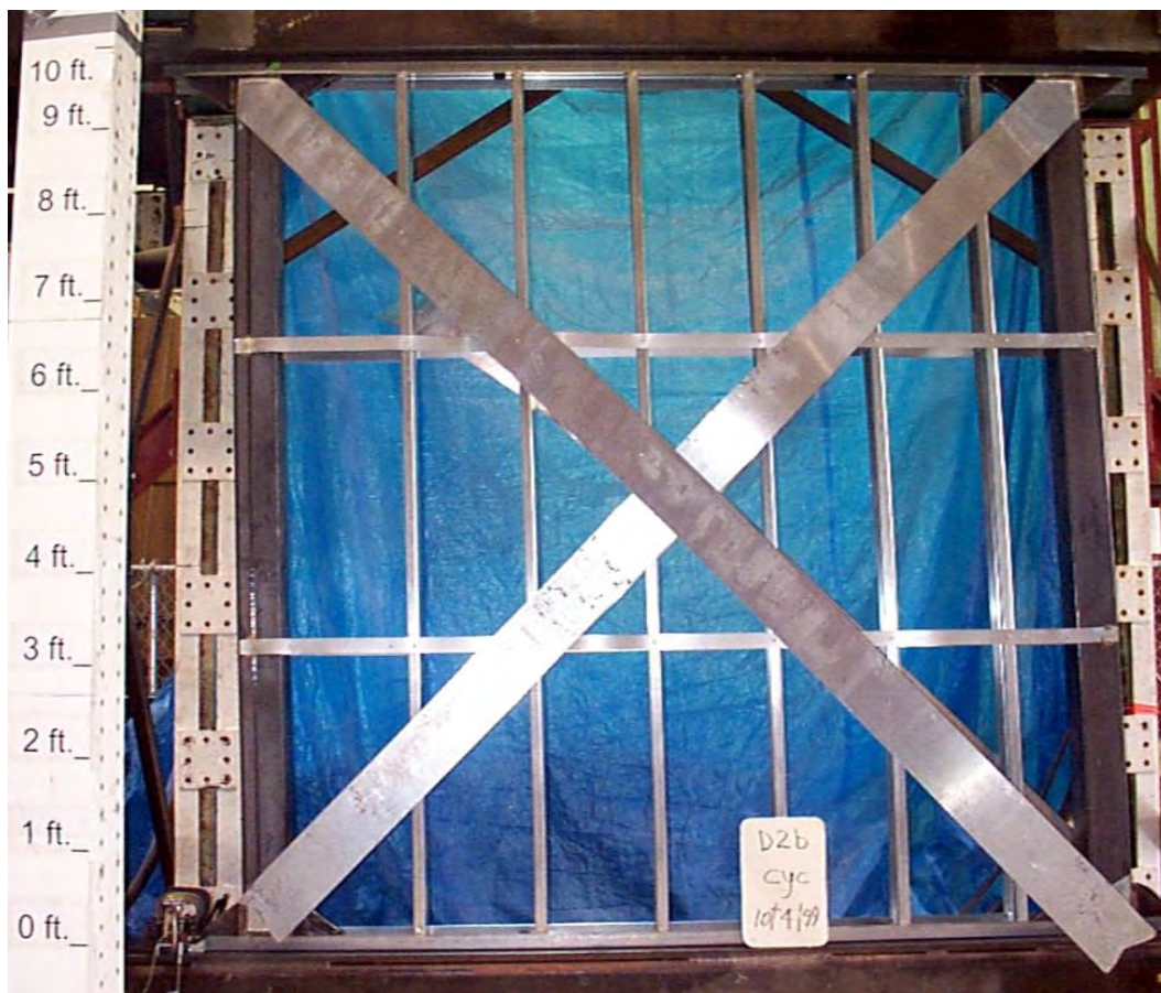
Figure 7-34. Overall view of the D2b test panel after the front strap failed at the bottom of the north (right) column at 2.6 in.
