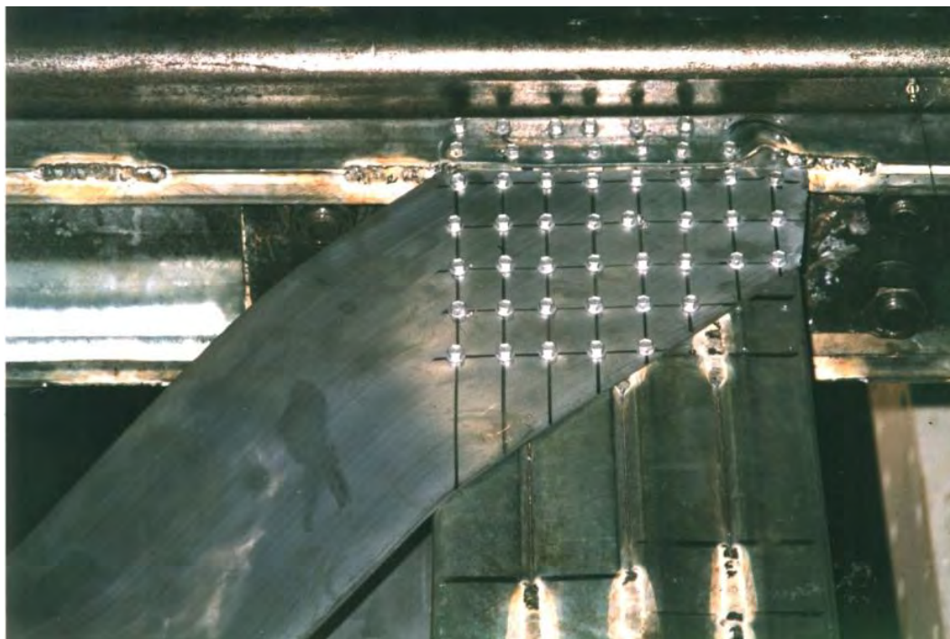
Figure 7-13. Top of north column showing buckled track after the A2b cyclic test.
