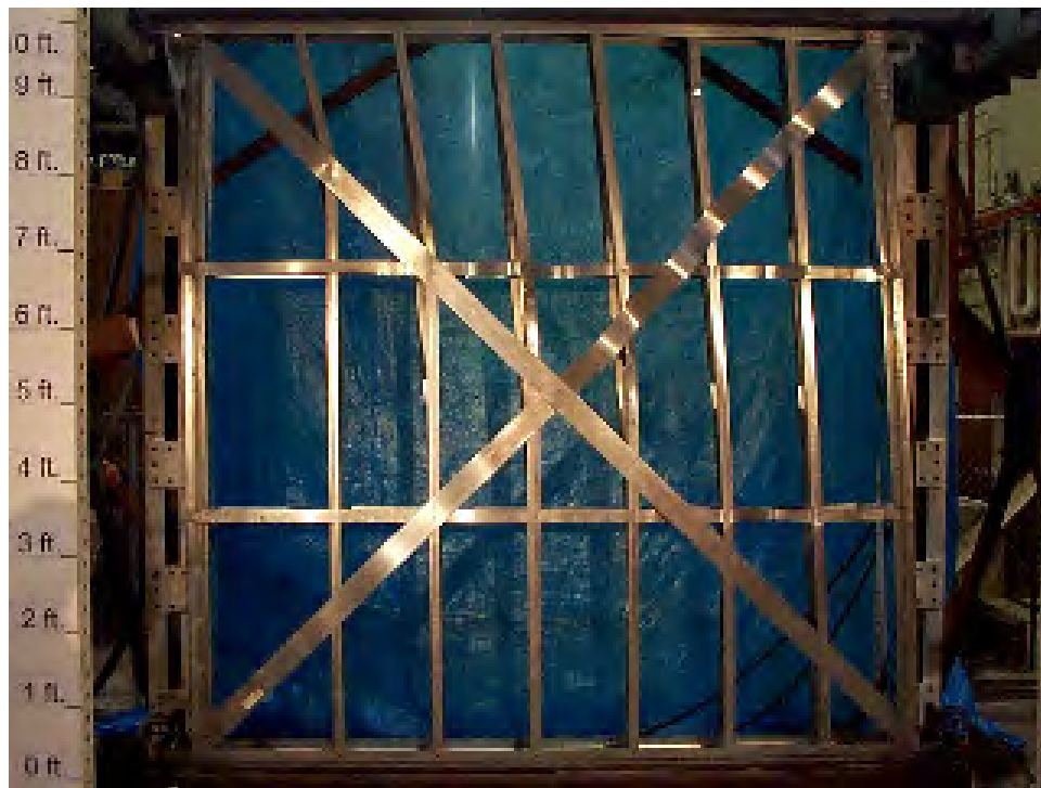
Figure 7-2. Overall view of failed A1a monotonically tested shear panel.
