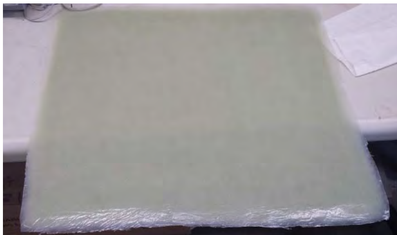
Figure 14. Composite panel after curing.
