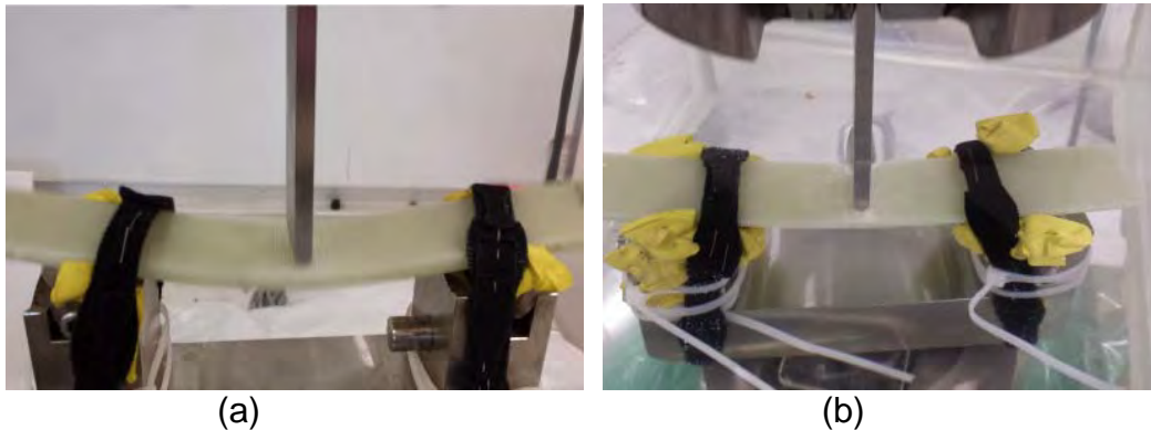
Figure 34. Signs of delamination of sample after initial loading in (a) air load (b) submerged water loading.
