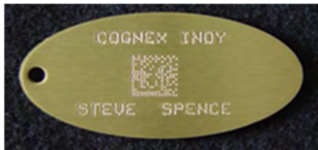
Figure 17. Dot Peening Example (from Spence, 2005).
