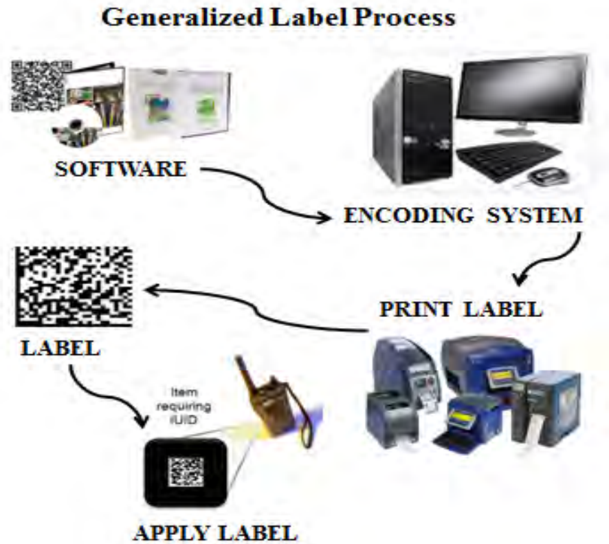
Figure 11. Generalized Label Process (after UID Forum, 2010).
