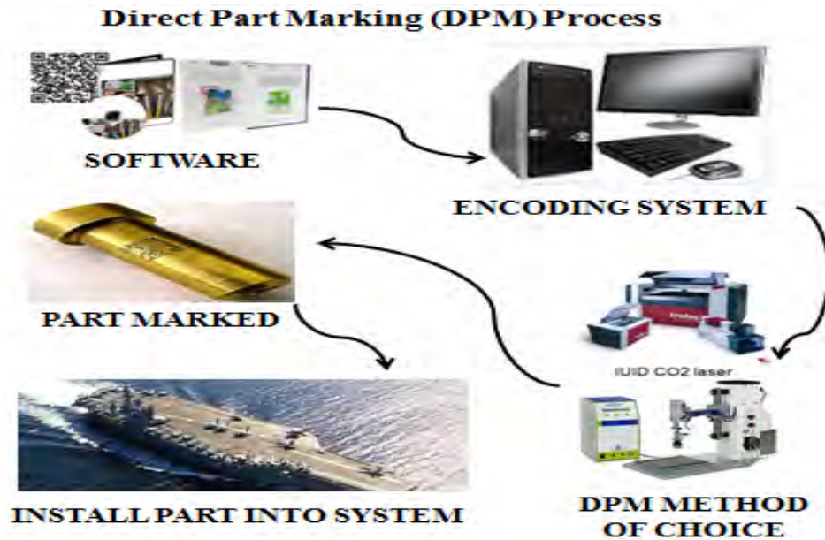
Figure 16. DPM Process (after UID Forum, 2010).
