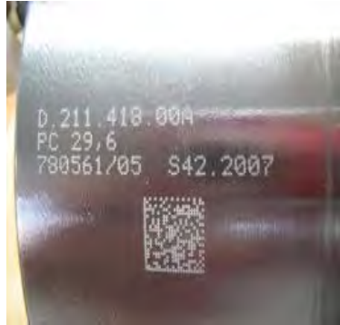
Figure 19. Laser Etching (from SIC Marking, 2014).
