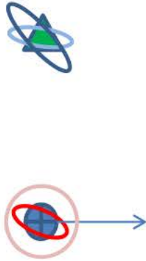
Figure 7. After two measurements of the same landmark, the robot's PUC, the red ellipse is substantially smaller than it was at the beginning. The initial ellipse is in light red to show the reduction. The updated uncertainty of the feature is shown as the light blue ellipse, and is markedly smaller than the initial, shown in dark blue.
