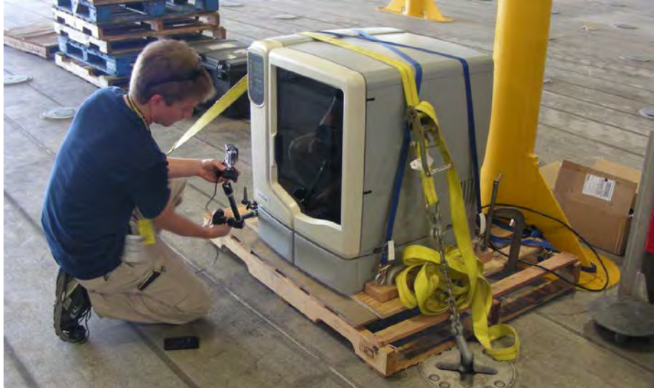
Figure 4. uPrint FDM machine on USNS Choctaw County (from Hess, 2014)
