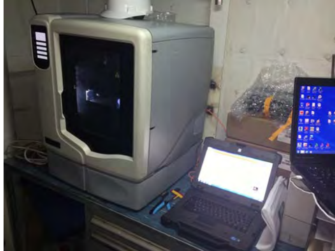
Figure 3. uPrint FDM machine in USS Essex machine shop (from Print The Fleet, 2013)
