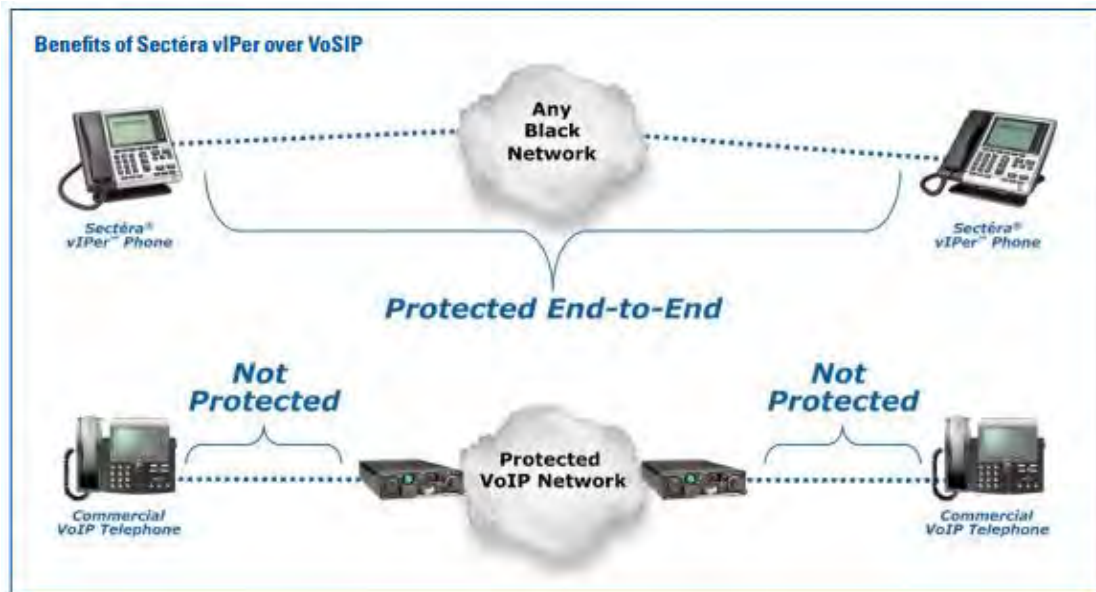
Figure 8. SVoIP vs. VoSIP Comparison, from [32]
