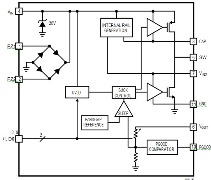
Figure 22. LTC3588-1 integrated circuit block diagram view (from [11]).
