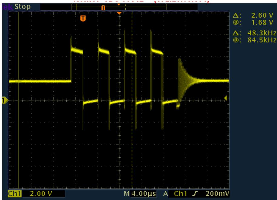
Figure 30. Buck chopper waveform measured from pin 5 shown in Figure 20.
