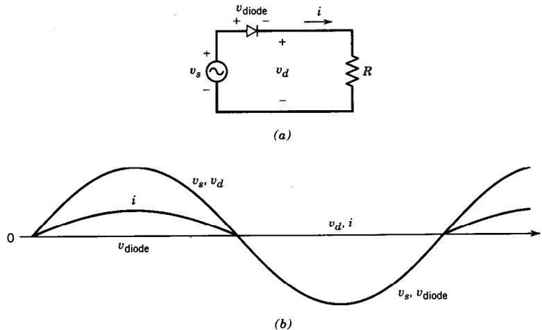
Figure 1. Simple diode rectifier circuit and waveforms (from [9]).
