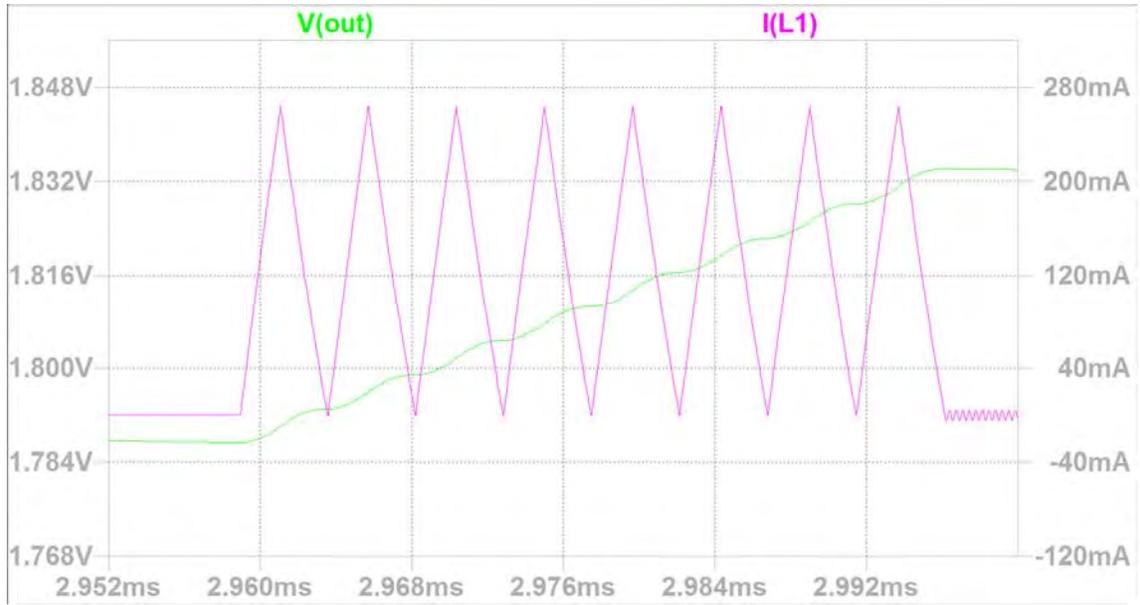
Figure 16. Simulated switching current waveform (measured through  $L_1$ ) and output voltage (measured at the  $V_{out}$  PIN) shown in Figure 11.
