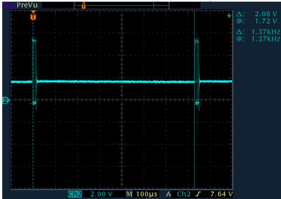
Figure 32. Chip voltage at pin 5 shown in Figure 20 with 500 Ω load. Ch2 shows 7.3 μs between pulses.
