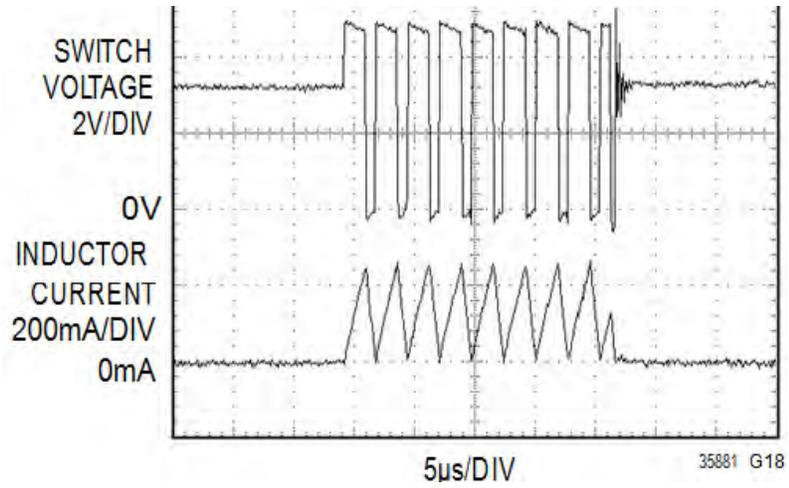
Figure 14. Switching waveform shown in the datasheet (from [11]).
