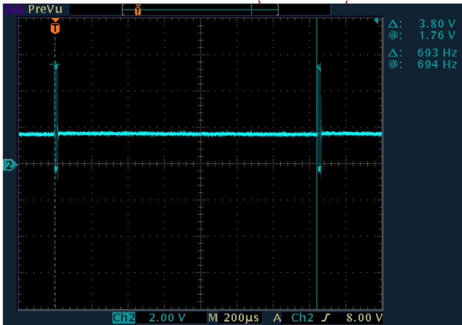
Figure 33. Chip voltage at pin 5 shown in Figure 20 with 1 kΩ load. Ch2 shows 1.43 ms between pulses.
