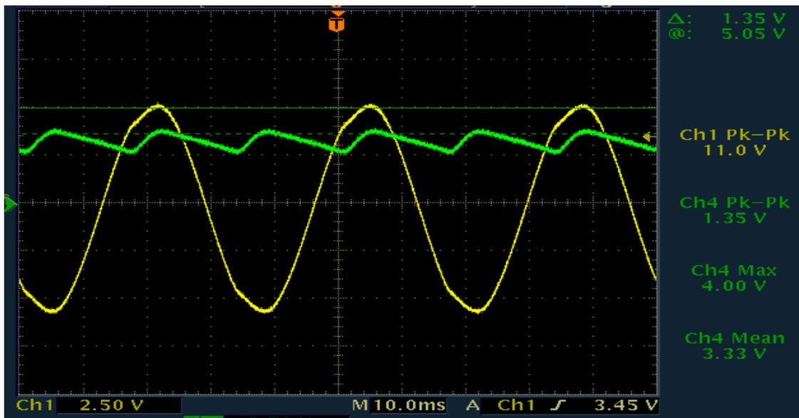
Figure 38. Rectification demonstration.
