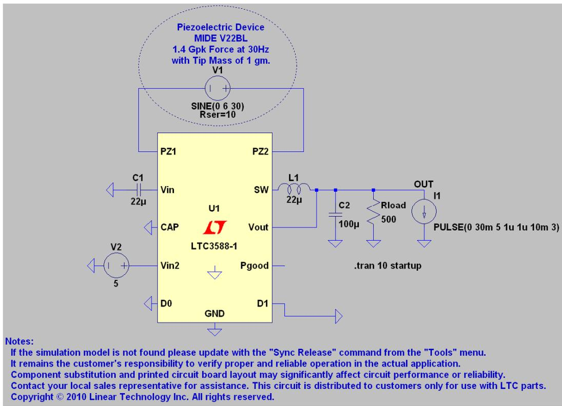
Figure 11. LTSpiceIV model of demonstration board (from [12]).
