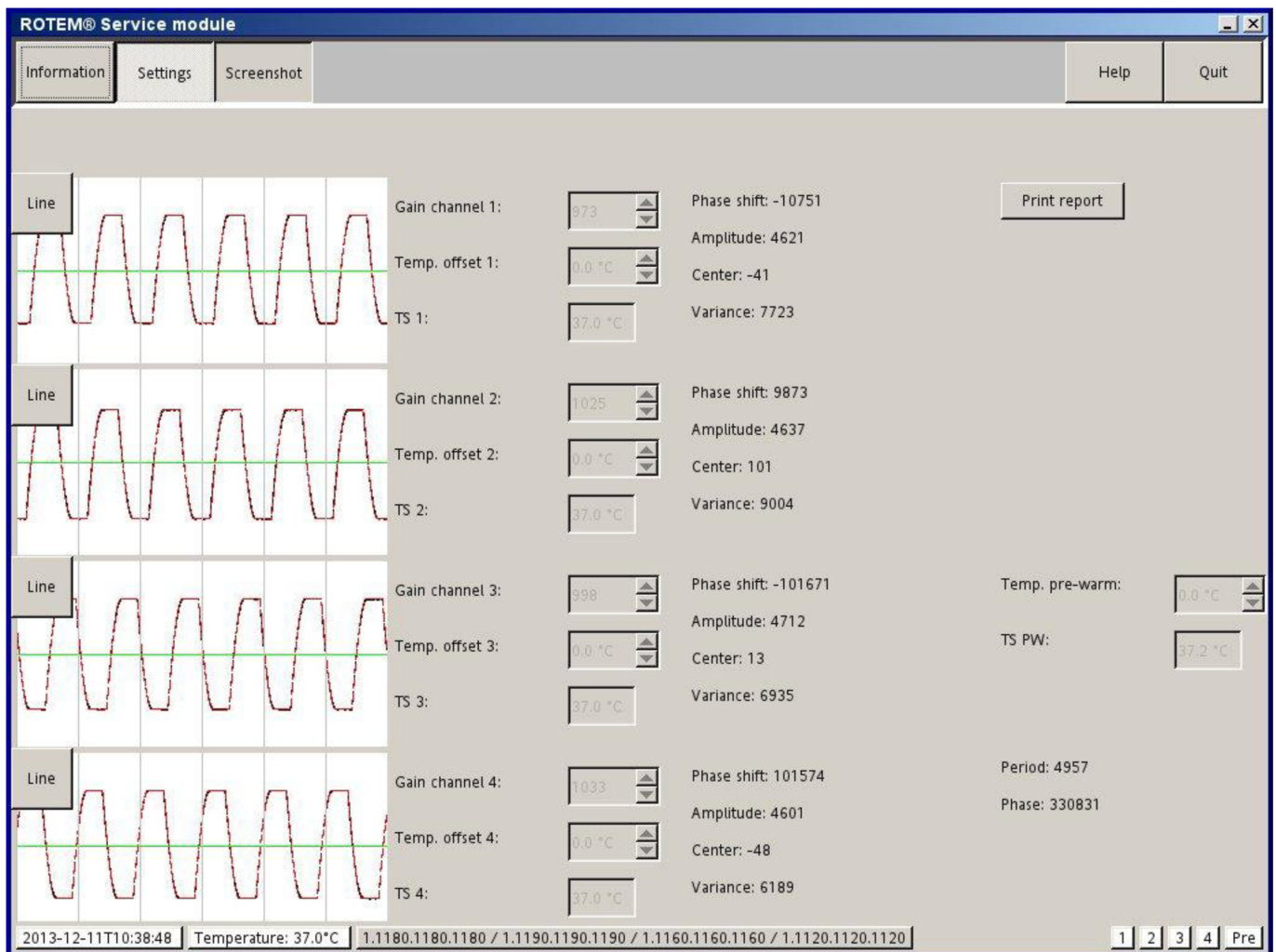
Figure 1. Control data of mechanical piston movement in the ROTEM machine during Sea State 3 with 4-m waves and 12-degree rolling of the ship. Red lines (actual rotation of the pistons) exactly overlay the calculated black lines.
