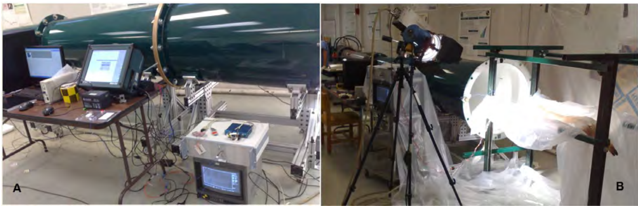
Figure 4. Swine shock tube testing setup. Figure A shows data acquisition system with the WSU conical extension in the background. Figure B shows the swine set-up for the swine test blast. The swine cadaver was suspended from a custom-built frame positioned in front of the shock tube.
