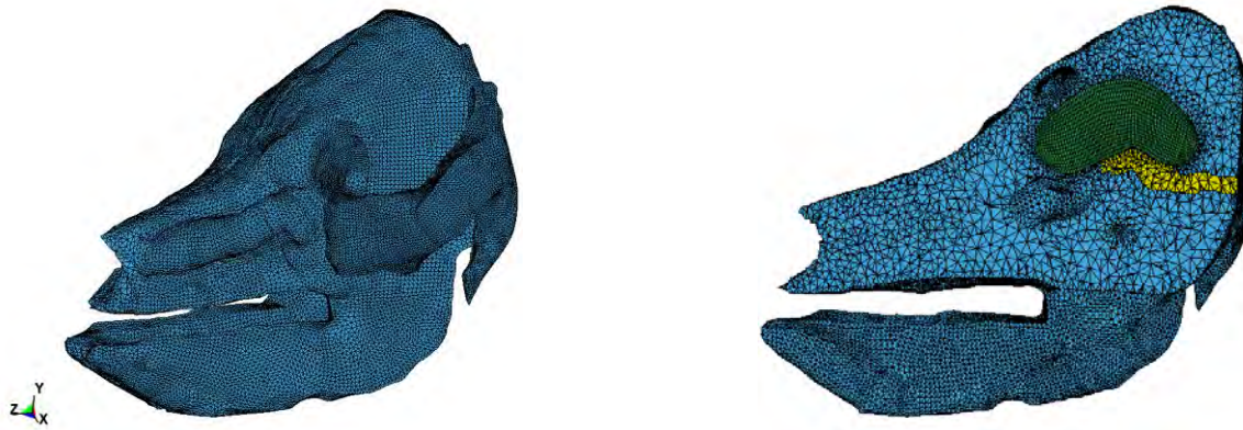
Figure 25. The pig head model with a tetrahedral mesh for the skull: (Left) Outside profile; (Right) Mid-sagittal view
