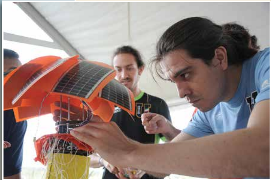
The 2014 CanSat competition, celebrating its 10-year anniversary, required teams to develop a soda-can-size satellite-type system (CanSat) capable of harvesting energy from the environment and transmitting telemetry in real time to a station on the ground.
