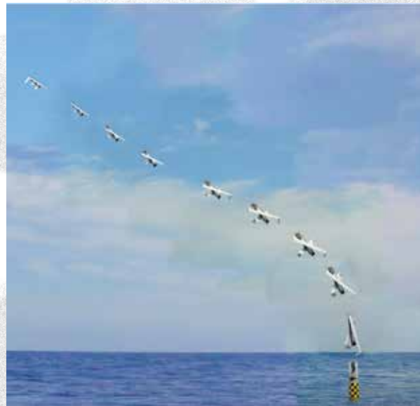
XFC UAS launch in time-lapsed photography. Deployed from the submerged submarine USS Providence , the XFC vertically launched from a Sea Robin launch vehicle (bottom right). The folding wing UAS autonomously deploys its X-wing airfoil and after achieving a marginal altitude, assumes horizontal flight configuration. (Photo: NAVSEA-AUTEC)
