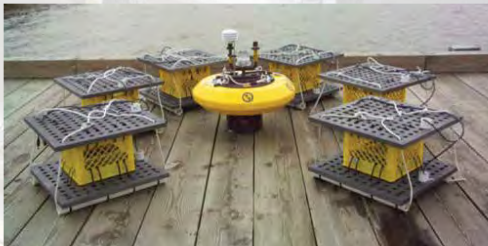
The combined power from six small-scale BMFCs was used to persistently operate a meteorological buoy (center) in the Potomac River. The buoy measured local weather conditions and transmitted data every five minutes to a land-based receiver.
