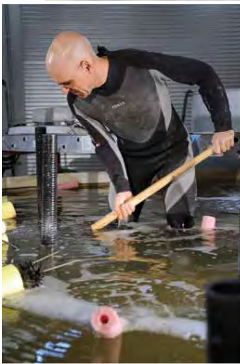
Dr. Leonard Tender (above, and with Marius Pruessner at right) working in the benthic mesocosm in the Laboratory for Autonomous Systems Research. The mesocosm contains 18 inches of seawater and 24 inches of synthetic marine sediment that has been inoculated with real marine sediment to provide necessary microbial activity. On the water surface are BMFC graphite bottlebrush cathodes; when deployed in the field, these cathodes are beneath the water surface but above the sediment surface. The vertical tubes indicate the locations of BMFC anodes embedded in the sediment.
