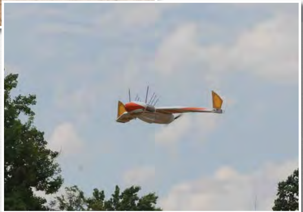
The Flimmer vehicle is an adaptation of NRL's WANDA for air-delivery.
