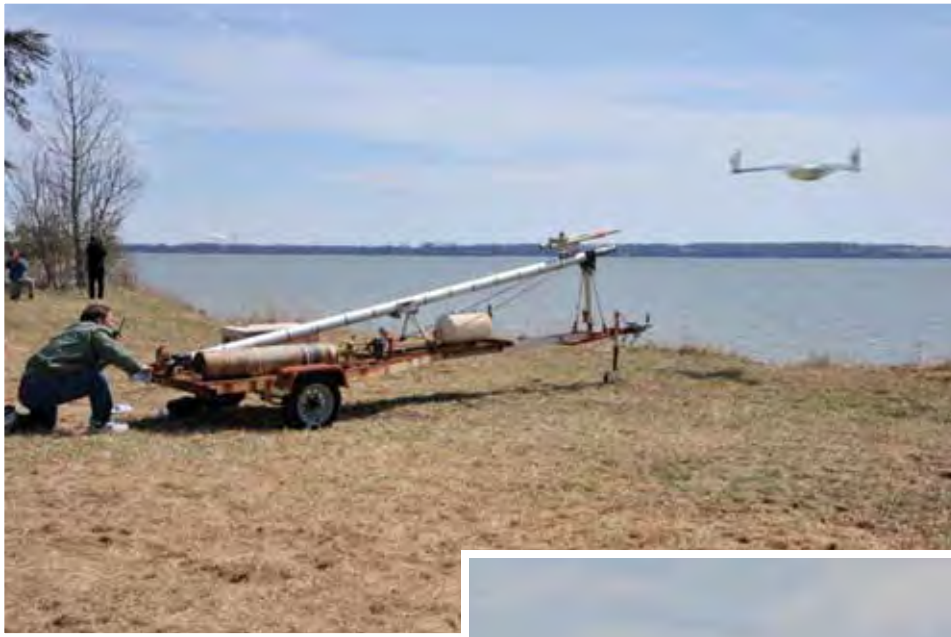
Flying WANDA takes flight, moments after departing the pneumatic launcher.
