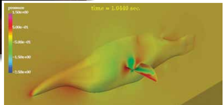
The geometry of the bird wrasse was modeled and computational fluid dynamics simulation was validated against experimental results.
