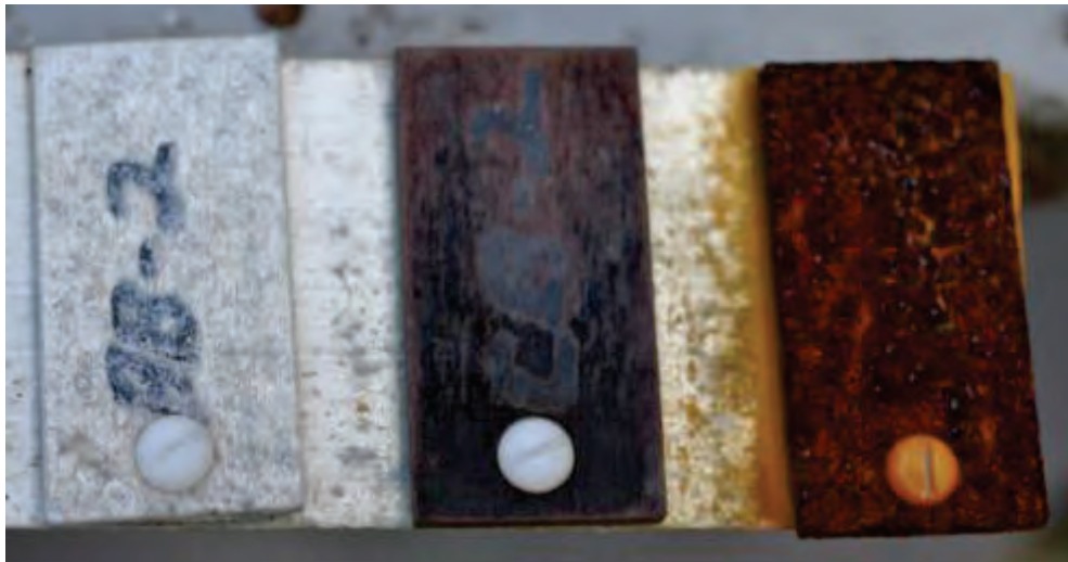
A 23. Rack 2, bare coupons at 12 months.
