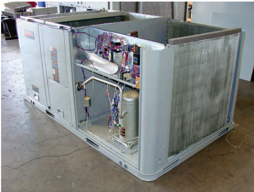
Figure 1. Interior layout of a Carrier-brand condenser, shown with coated fins.
