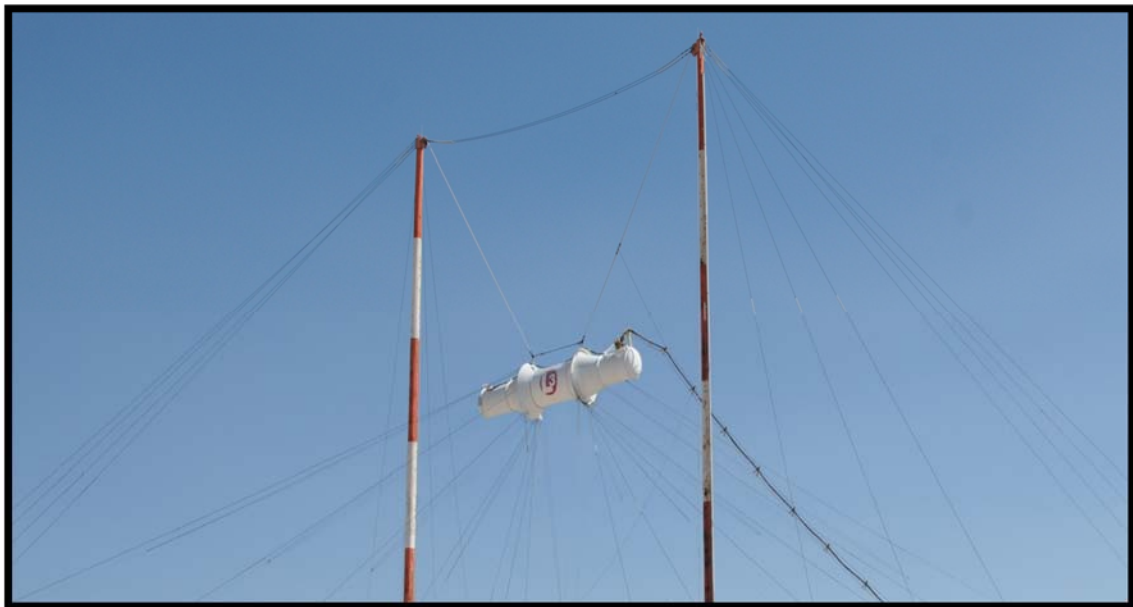
Figure 2. WSMR AFEMP Pulser and Antenna.
