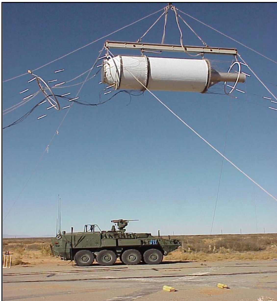
Figure C-1. Generic missile launcher HEMP test setup.
