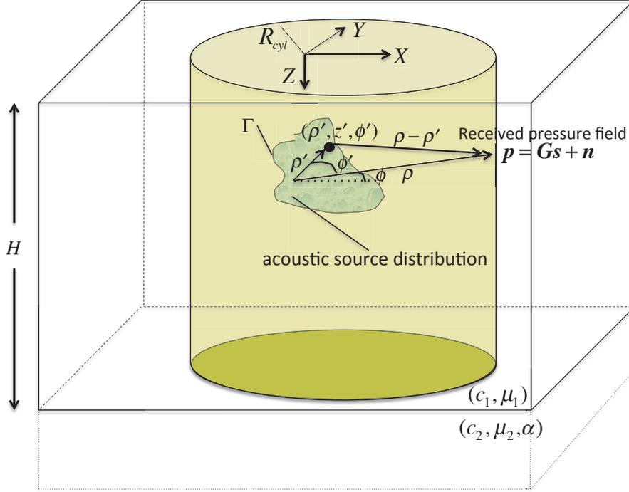
Fig. 1 — Waveguide configuration and cylindrical coordinate system used to evaluate the acoustic field and capacity on a cylindrical surface exterior to an arbitrary source distribution
