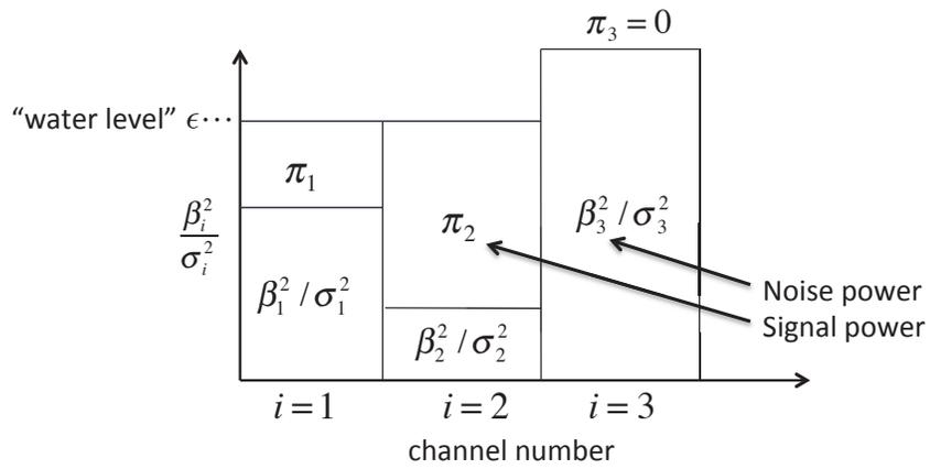
Fig. 4 — Illustration of the waterfilling procedure used to evaluate Eq. (22)
