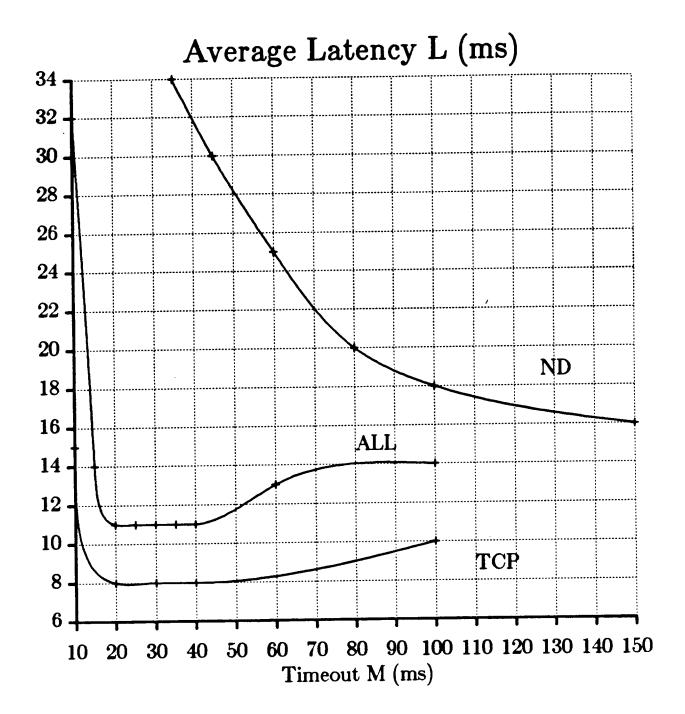
Figure 8.  $L \ {\it versus} \ \emph{M} \ {\it for various traces (other factors at nominal levels)}$
