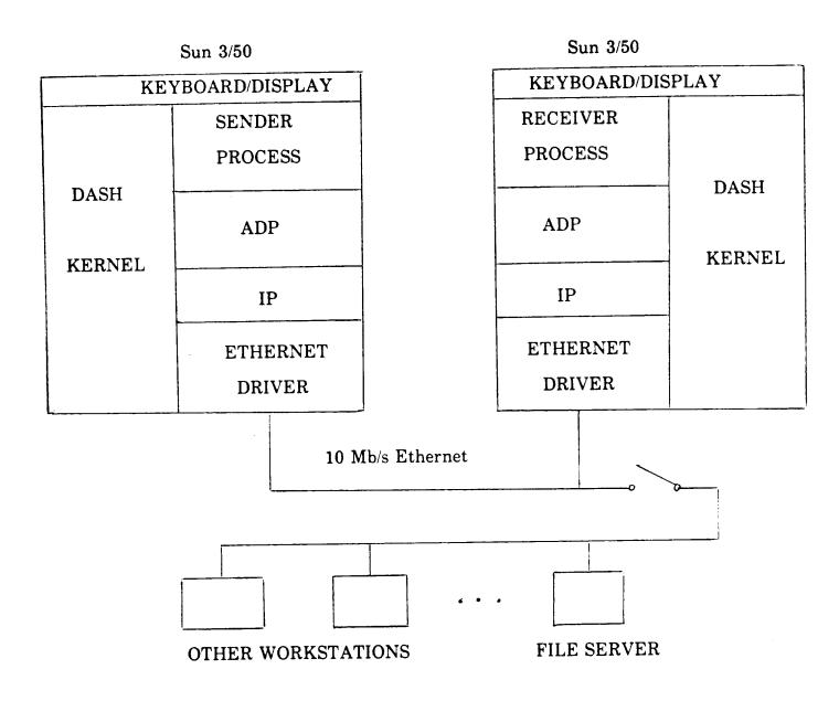
Figure 3. The experimental setup.
