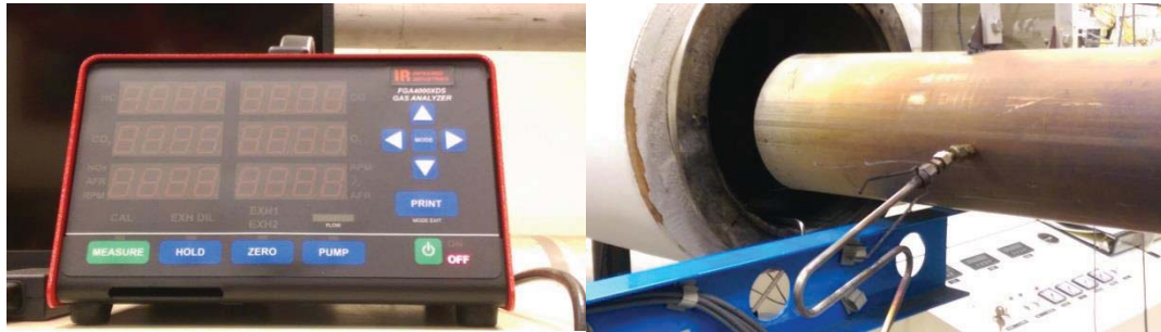
Figure 21: Five Gas Analyzer with exhaust port location
