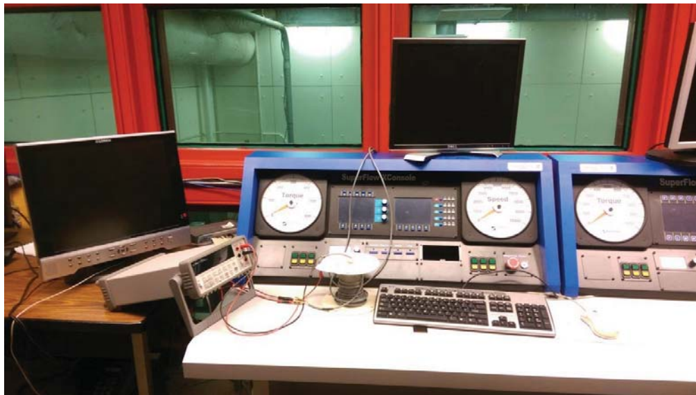
Figure 23: SuperFlow TM control console with multimeter
