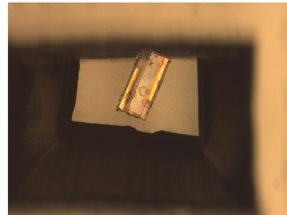
Single xfab device picked up on PDMS stamp
