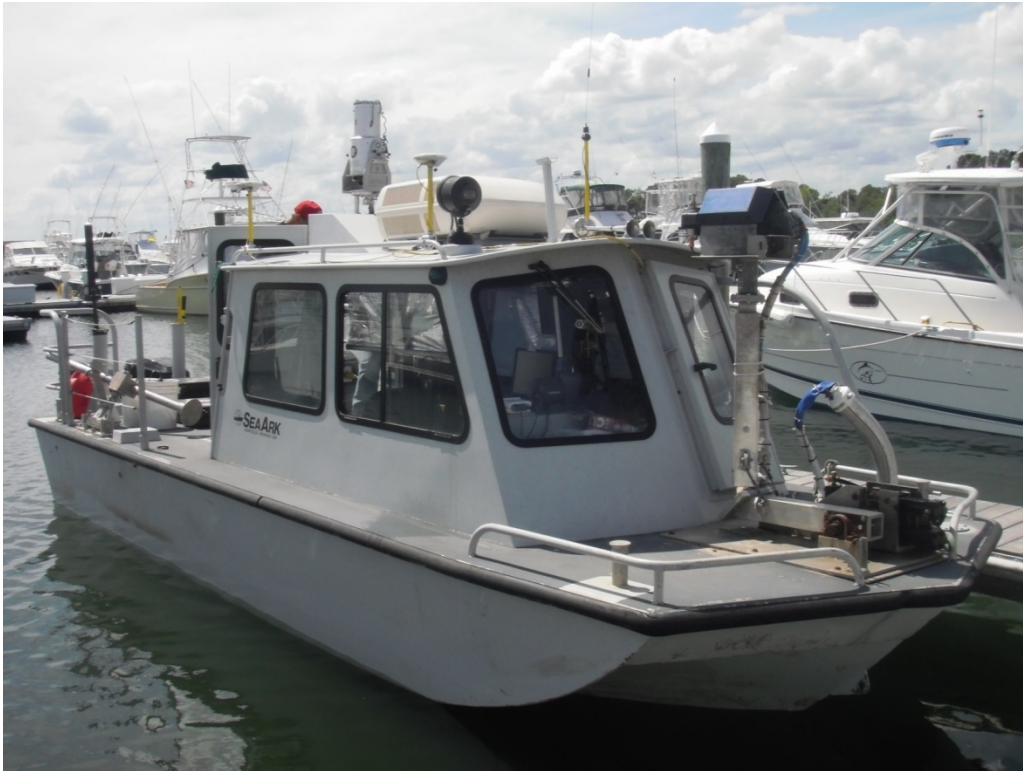
Figure 2.13. Bathymetric survey boat.
