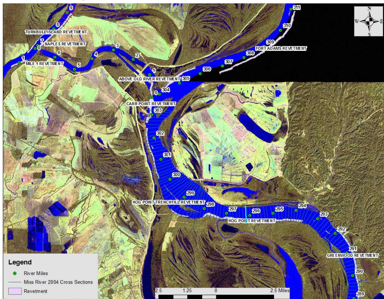
Figure 4.6. Mississippi River revetments and cross section locations.
