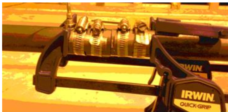
Figure 46. The contact between two rods imitating the crack.
