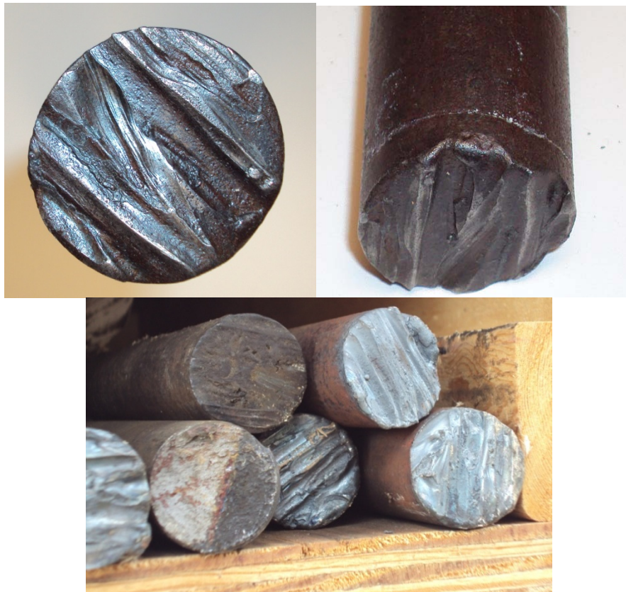
Figure 21. Torch-cut rod ends.
