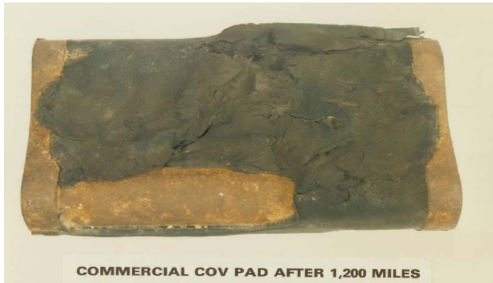
Fig. 2 Typical commercial pad failure mode
