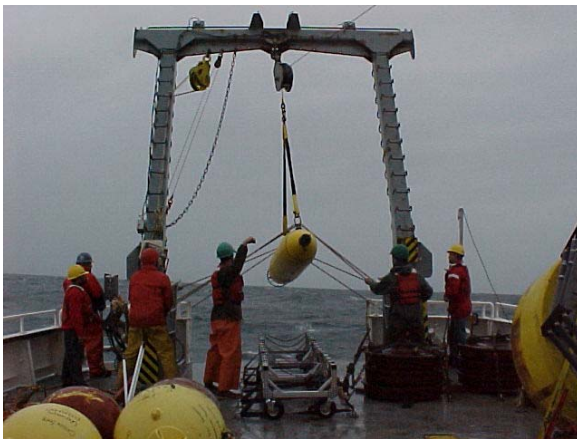
Figure 2: Deployment (right) and retrieval (left) of AUV from R/V Wecoma off the coast of Oregon, March 19, 2003.
