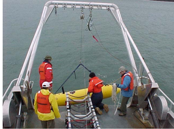
Figure 1: AUV with full payloads. Getting ready to perform a compass calibration in Homer, Alaska (left panel). Deployment of AUV from OSU's 54' long R/V Elakha in the Yaquina Bay during acceptance trials (right panel).
