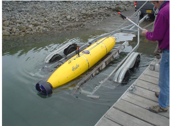
Figure 3: Deployment of AUV by lowering a boat trailer in a boat ramp (right panel) in Kachemak Bay, Homer, Alaska. AUV steaming at the surface in the Kachemak Bay on June 2, 2003.
