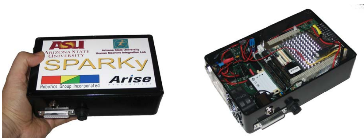
Figure 1: A PC104, motor amplifier, communication board, fan, and power converter were mounted in a small box to be worn by the user. The batteries are mounted separately from the box.
