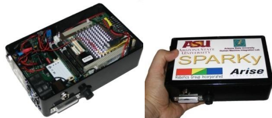
Fig. 9. The computer and electronics are packaged in a small portable package for this phase of SPARKy. SPARKy II will include a microprocessor and electronics embedded in the prosthesis.
