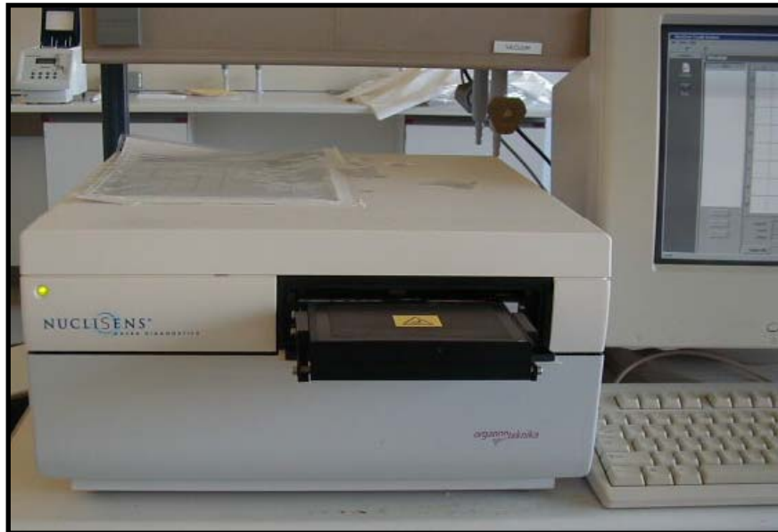
Figure 3. Nuclisens EasyQ Reader that detects NASBA amplification in Real Time.
