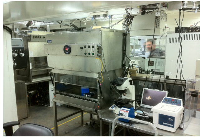
Figure 6-6: The Heavy Laboratory Engineering Controls Include Fume Hood, Class II Biosafety Cabinet and Glovebox.
