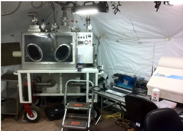
Figure 6-6: The Heavy Laboratory Engineering Controls Include Fume Hood, Class II Biosafety Cabinet and Glovebox.
