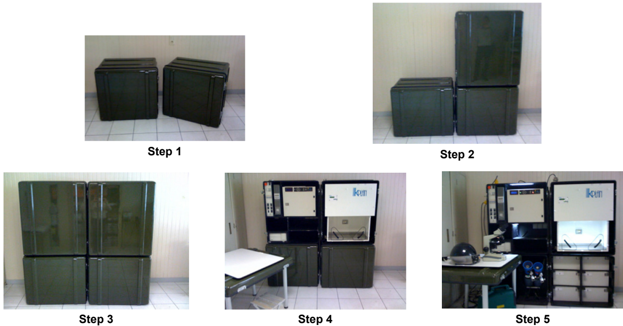
Figure 3-3: The Laboratory's 5 Step Assembly.
