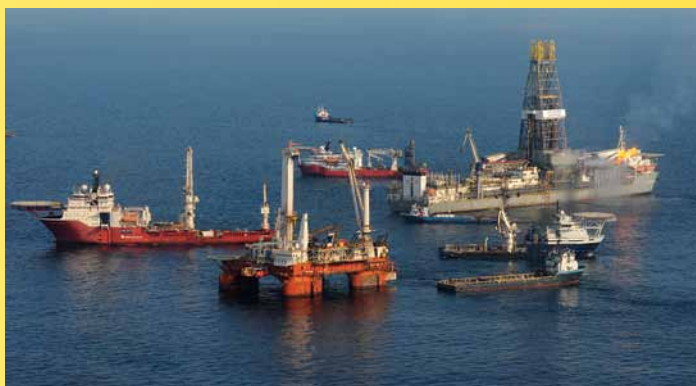
A mobile offshore drilling unit holds position directly over the damaged Deepwater Horizon blowout preventer as a drillship burns gas brought to the surface through a tube placed into the ruptured drill pipe. U.S. Coast Guard photo by Petty Officer Patrick Kelley.
