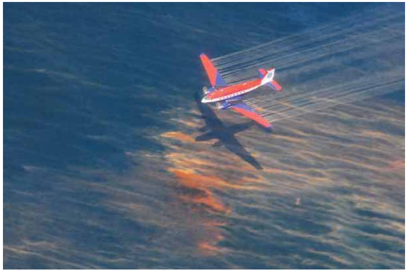
The crew of a Basler BT-67 fixed-wing aircraft applies dispersants to an oil slick during the Deepwater Horizon response. U.S. Coast Guard photo by Petty Officer Stephen Lehmann.
